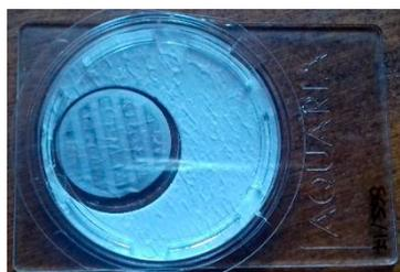
**Figure 4.** Example of filter sampled at University of Florence for insoluble EC/OC/TC measurements in melted snow.
