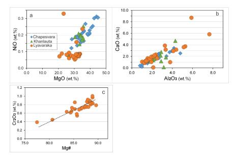
**Figure 13.** (**a**–**c**). Plot of contents of MgO vs. NiO in wt.% (**a**),  $Al_2O_3$  vs. CaO in wt.% (**b**), and values of the Mg# vs. contents of  $Cr_2O_3$  in wt.% (**c**), in ultrabasic rocks of the Lyavaraka complex (orange symbols), compared with the Chapesvara sill [12] (blue diamonds) and the Khanlauta differentiated flow [13] (green triangles).
