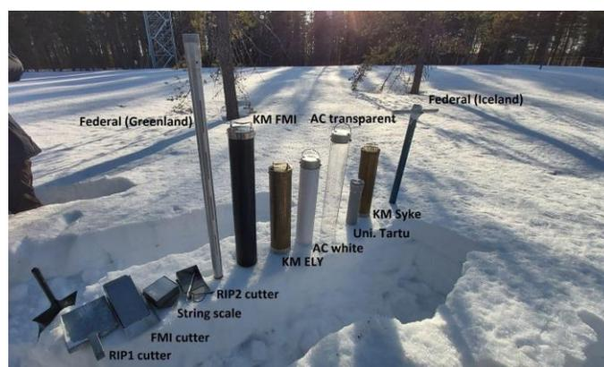
**Figure 1.** The tube samplers and density cutters used in the study.
