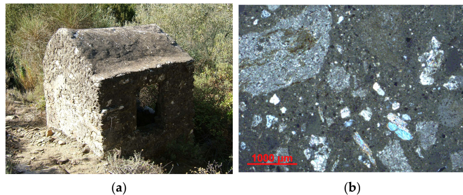
Figure 12. (a) “Palmento”, masonry structures of modest dimensions for the pressing of grapes, from where mortar samples were taken. (b) Bedding mortar of a “palmento” with dolostone and marble fragments in the aggregate (image at the optical microscope in thin section, crossed polarised light).
