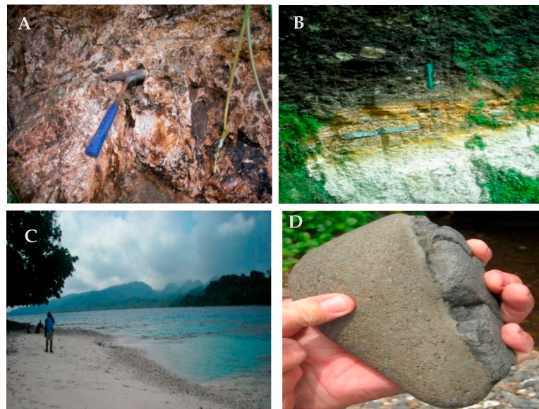
Figure 6. Field images of Ambitle Island deposits and geomorphology. (A) Volcanogenic oxidized siltstone at Niffin. (B) Pyroclastic deposit at Niffin River. Weathered mafic matrix-supported pyroclastic lapilli-block tuff deposit unconformably overlying horizontal ash-clay bed (base surge) and quartz-pumice-rich felsic ignimbritic layer. (C) Eastern side of Ambitle characterized by steep volcanic domes. Image taken from eastern point of Babase Island. (D) Vesicular feldspar–pyroxene phyric basaltic float containing a mafic or basaltic xenolith.
