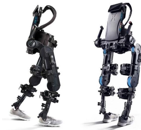
**Figure 3.** Powered lower-limb exoskeleton ExoAtlet II from ExoAtlet Global SA, Luxembourg. Adapted with permission from [23]. Copyrighted by ExoAtlet, 2019.
