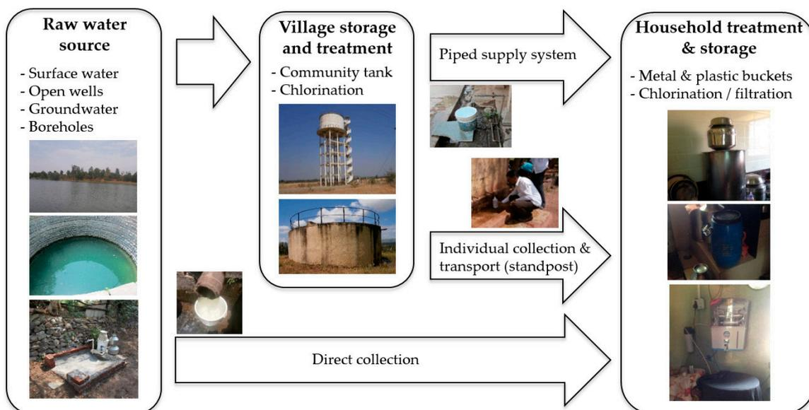
Figure 2. Water supply and treatment system. Pictures taken by article authors.
