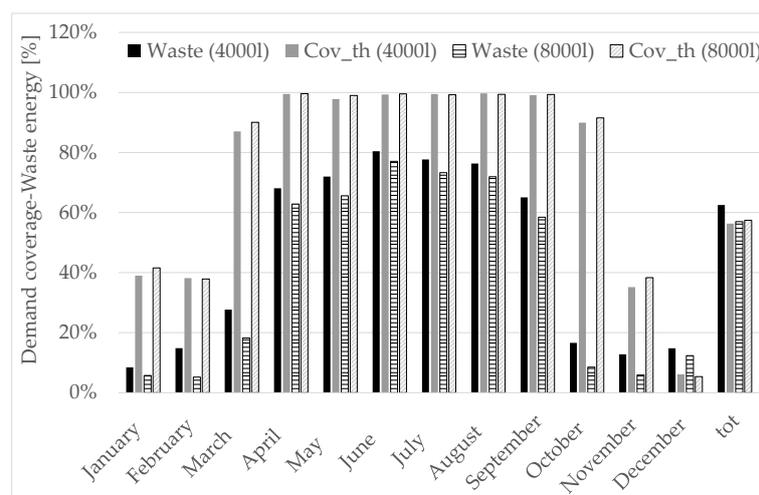
**Figure 5.** Monthly thermal energy wasted and total energy demand coverage for the case of a terraced house in Ancona with a thermal energy storage (TES) volume of 4000 L (standard configuration) and with a TES volume of 8000 L (double size compared to the standard configuration).
