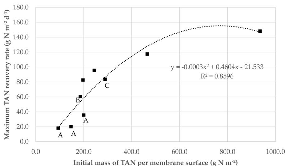
**Figure 3.** Maximum recovery rates in the literature studies and in the present study using GPM technology for N recovery vs. the ratio of initial mass of TAN in wastewater per membrane surface. A second order equation and R<sup>2</sup> are represented: (A) García-González and Vanotti [15]; (B) García-González et al. [14]; (C) García-González et al. [24]. Values of the present study are presented as symbols without letters.
