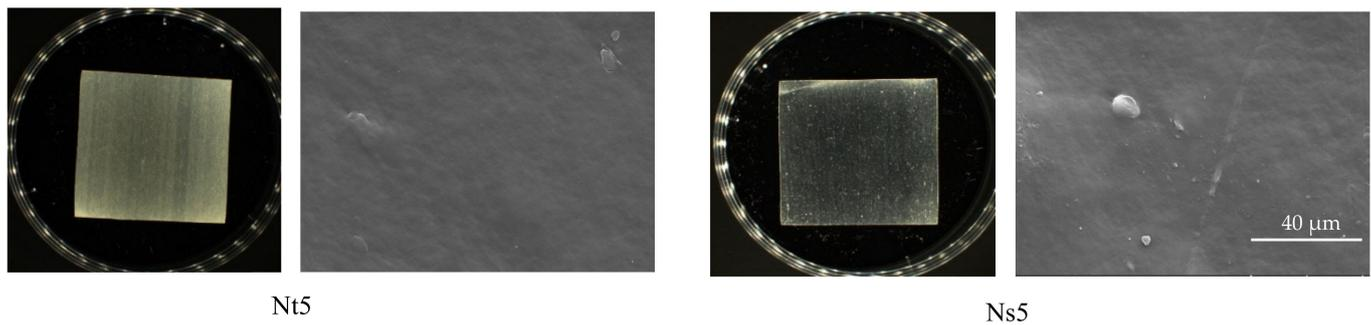
**Figure 1.** Sample images (real photos and photos taken with a scanning electron microscope-SEM, Hitachi SU 8010, Tokyo, Japan). Abbreviations: 0- pure LDPE; Nt 1,3,5 (samples with 1%, 3% and 5% Natamax<sup>®</sup>); Ns 1,3,5 (samples with 1%, 3% and 5% Nisaplin<sup>®</sup>).
