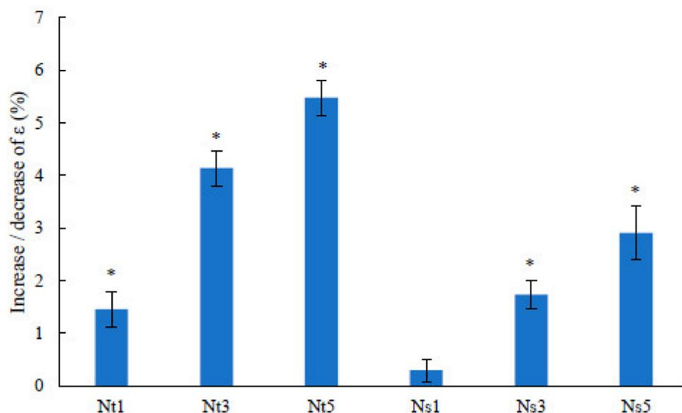
**Figure 3.** Elongation at break (percentage differences compared to samples without biocide). Statistically significant differences ( $p < 0.05$ ) compared to the control (0) are marked with asterisks. Abbreviations: as in Table 1.
