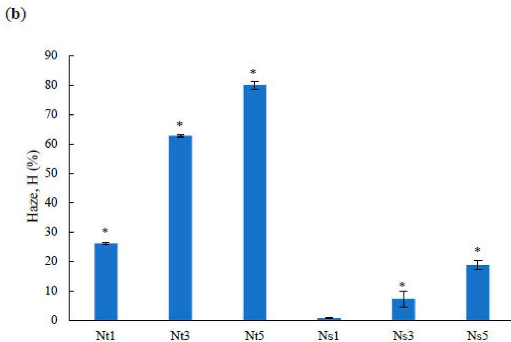
**Figure 4.** Optical properties (percentage differences compared to samples without biocide): (a) transparency; (b) haze. Statistically significant differences ( $p < 0.05$ ) compared to the control (0) are marked with asterisks. Abbreviations: as in Figure 1.
