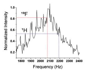
**Figure 2.** Instrument response of the tuned circuit used for detection of the fluorobenzene compounds without a sample. The blue dotted line corresponds to the center frequency of the  $^{1}$ H nucleus, while the red dotted line denotes the  $^{19}$ F response. The  $^{19}$ F resonances are preferentially enhanced, relative to  $^{1}$ H by a factor of 1.52. The 60 Hz overtone noise spikes were omitted for clarity.
