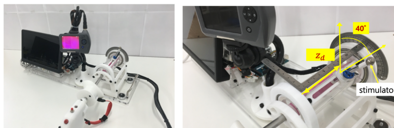
Figure 7. Design for the testbed based on 3D printing technology to confirm two main points: (a) safe insertion and (b) exact measurement.
