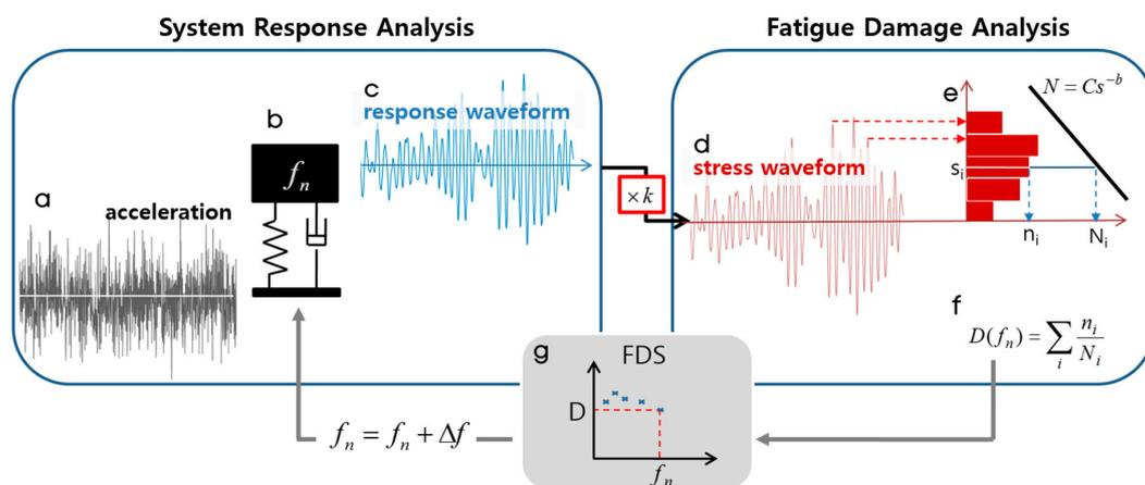
**Figure 1.** Flowchart of fatigue damage spectrum (FDS) calculations, (a) input acceleration, (b) Single Degree of Freedom (SDOF) system which is the virtual specimen, (c) velocity response, (d) stress waveform which is obtained by multiplying  $k$  to the velocity response, (e) stress counting and idealized stress–number (S-N) curve, (f) accumulation of damage index, (g) FDS.
