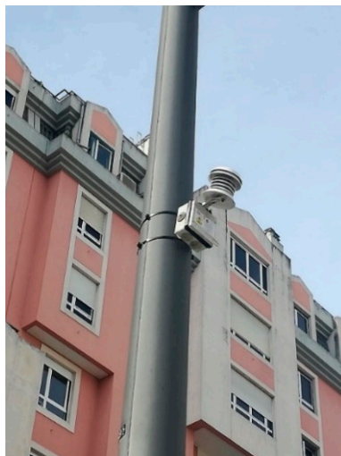
Figure 3. Thermo-hygrograph (Hobo No 3—see Figure 3) in Telheiras.
