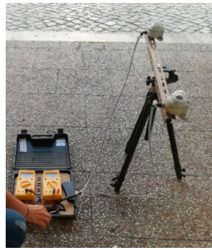
Figure 5. The radiation measurement system composed by a pyranometer and a pyrgeometer.
