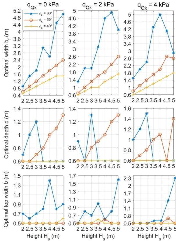
Figure 8. Optimal design for  $k = 2/3$ ,  $\beta = 20^\circ$  and  $\gamma = 18 \text{ kN/m}^3$ .
