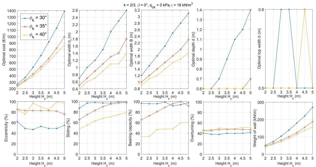
**Figure 2.** The optimal design of a gravity retaining wall for soil-wall interaction coefficient  $k = 2/3$ , slope angle  $\beta = 0^\circ$  and variable surcharge load  $q_{Qk} = 0$  kPa.
