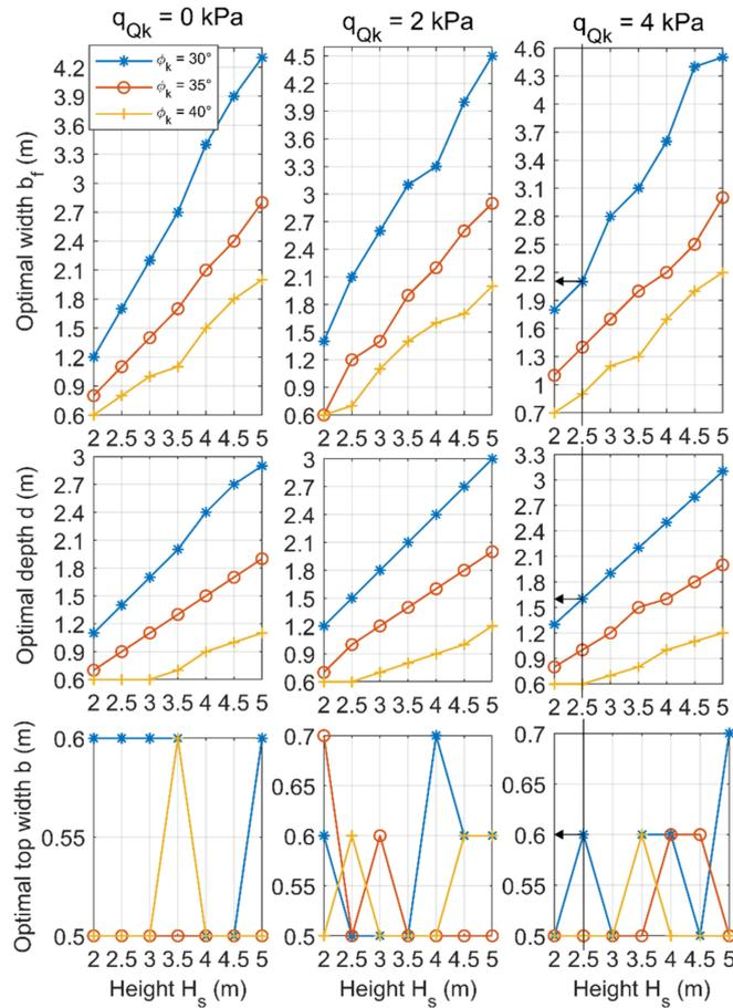
**Figure 3.** Optimal design for  $k = 0.5$ ,  $\beta = 20^\circ$  and  $\gamma = 18$  kN/m<sup>3</sup>.
