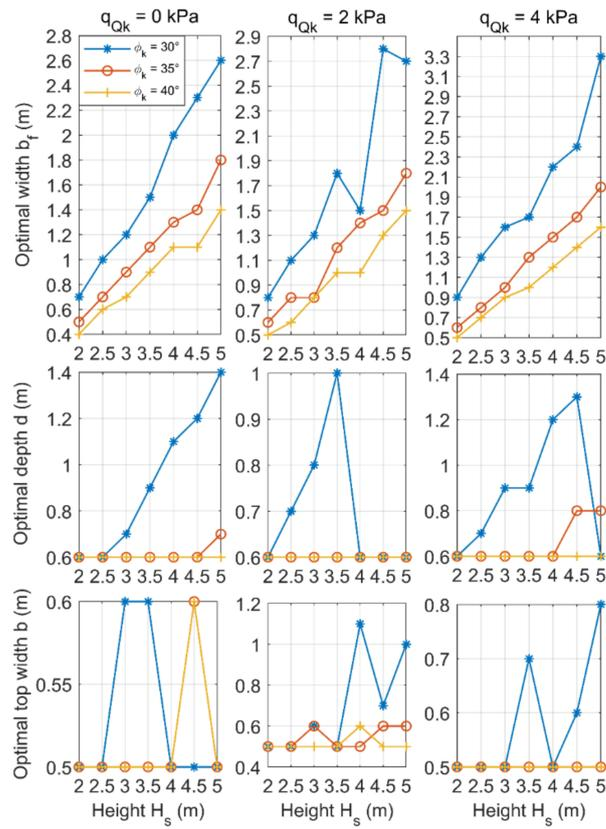
Figure 6. Optimal design for  $k = 2/3$ ,  $\beta = 0^\circ$  and  $\gamma = 18 \text{ kN/m}^3$ .
