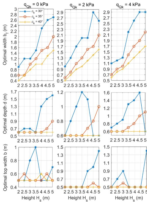
Figure 7. Optimal design for  $k = 2/3$ ,  $\beta = 10^\circ$  and  $\gamma = 18 \text{ kN/m}^3$ .
