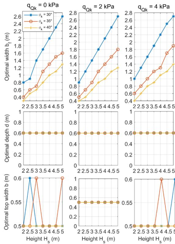
Figure 10. Optimal design for  $k = 1$ ,  $\beta = 10^\circ$  and  $\gamma = 18 \text{ kN/m}^3$ .
