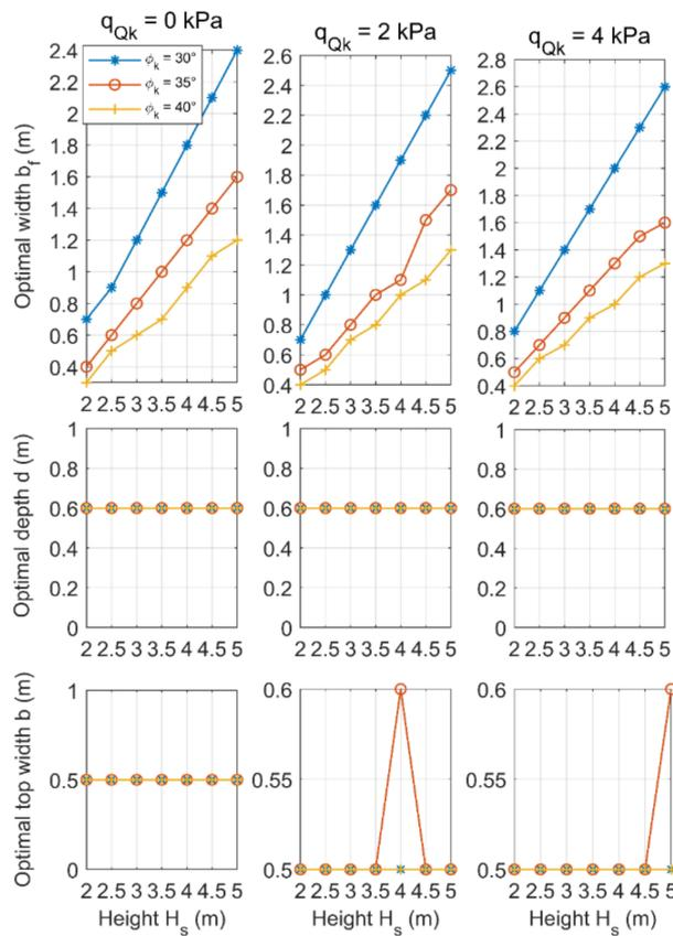
Figure 9. Optimal design for  $k = 1$ ,  $\beta = 0^\circ$  and  $\gamma = 18 \text{ kN/m}^3$ .
