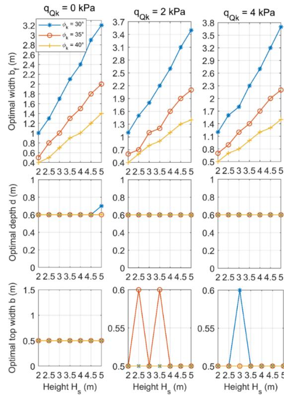
Figure 11. Optimal design for  $k = 1$ ,  $\beta = 20^\circ$  and  $\gamma = 18 \text{ kN/m}^3$ .
