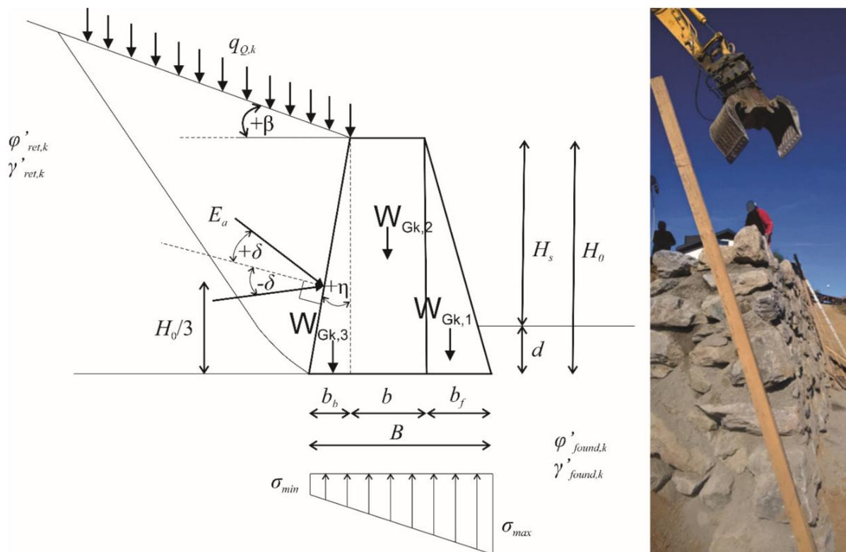
Figure 1. Geometry and parameters of a gravity retaining wall.
