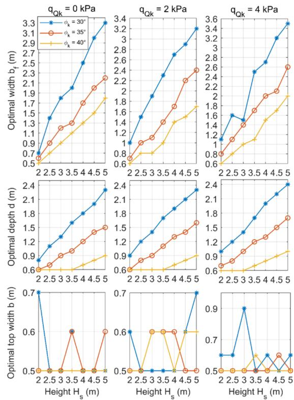
Figure 5. Optimal design for  $k = 0.5$ ,  $\beta = 10^\circ$  and  $\gamma = 18 \text{ kN/m}^3$ .
