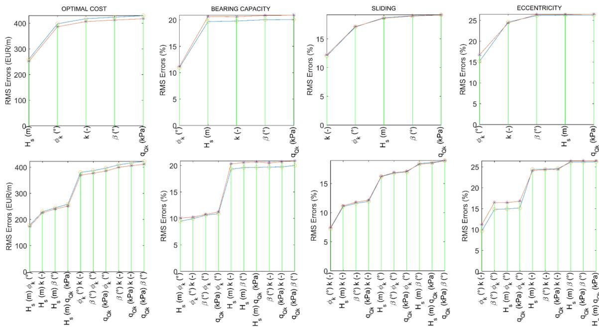
**Figure 12.** Influence of each input variable on the optimal cost of a gravity retaining wall and the utilization of geotechnical conditions.
