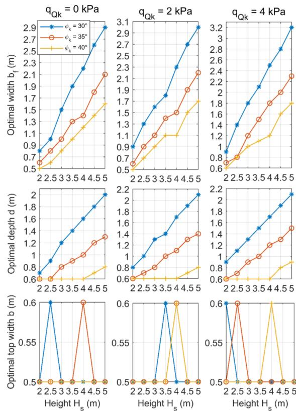
Figure 4. Optimal design for  $k = 0.5$ ,  $\beta = 0^\circ$  and  $\gamma = 18 \text{ kN/m}^3$ .
