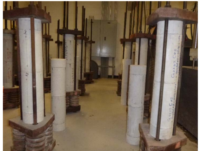
Figure 3. Creep test setup and specimen dimensions (25 mm = 1 in.).
