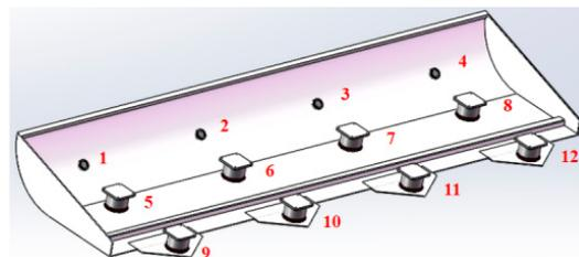
Figure 5. Pressure sensor installation location.
