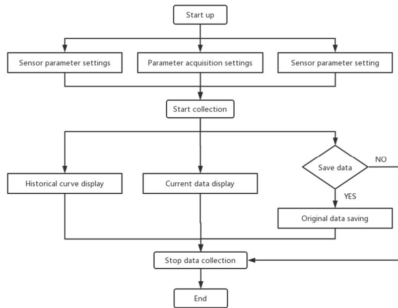
Figure 4. Flow chart of measurement system software.
