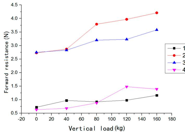
Figure 17. Relationship between forward resistance and vertical load.
