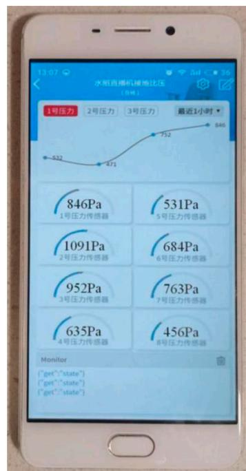
Figure 10. Internet of things measurement system—mobile terminal.
