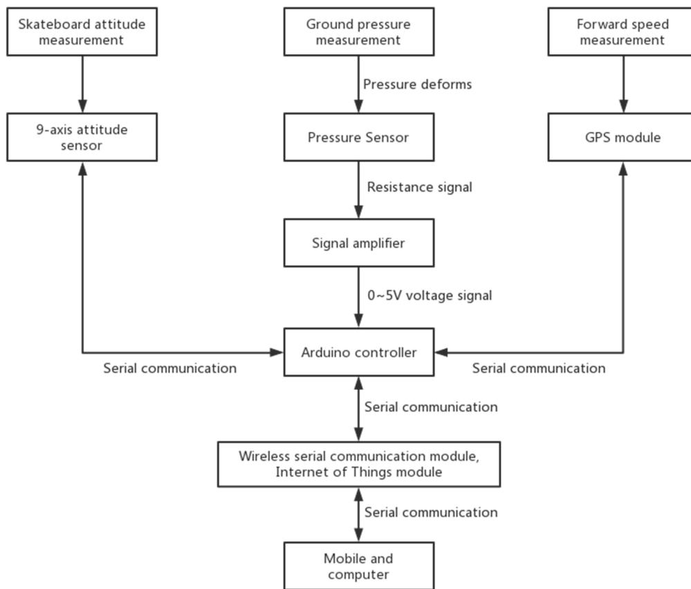
Figure 3. Flow chart of ground pressure measurement system.
