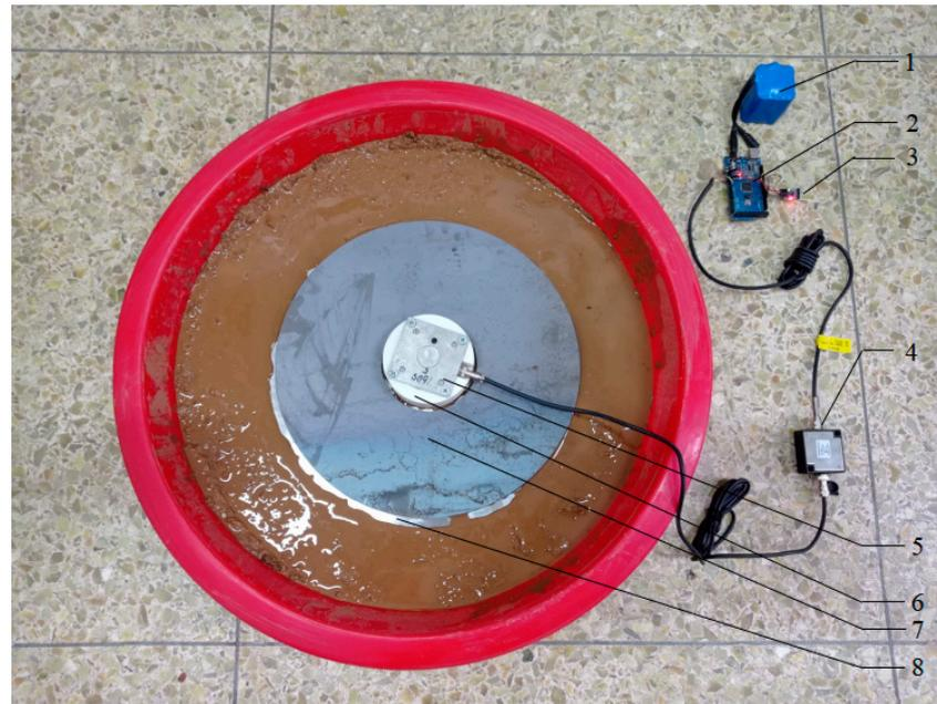
**Figure 7.** Ground pressure calibration device. 1. 12 V power supply. 2. Arduino controller. 3. Wireless serial port transceiver module. 4. Signal amplifier. 5. Pressure sensor. 6. Mounting base. 7. Counterweight plate. 8. Bottom plate.
