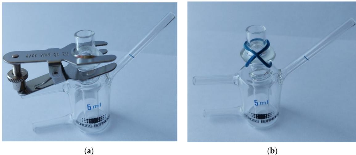
**Figure 5.** (a) Standard Franz cell with metal clip; (b) Franz cell fastened with an elastic band suitable for application with alternating magnetic field.
