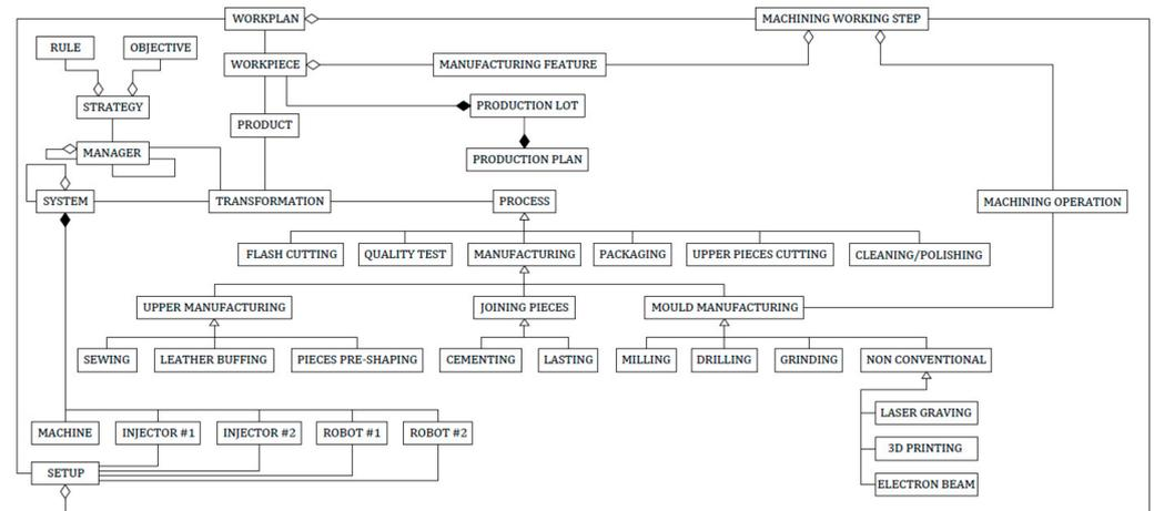
**Figure 3.** Class diagram of the conceptual reference framework.
