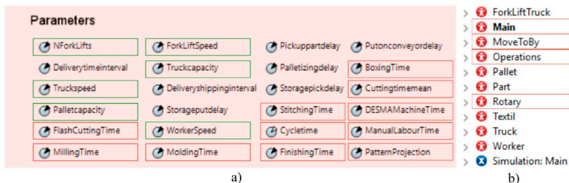
**Figure 4.** (a) System parameters (with a green frame the parameters that represent agent characteristics are outlined while parameters framed in red represent the main times of the system). This representation is associated with the direct-injection process. (b) Agents defined (agents framed in red are necessary in order to store logical blocks). These agents are associated with the direct-injection process.
