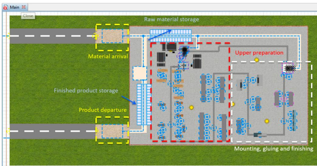
**Figure 9.** Spatial representation of the mounting-and-cementing process.
