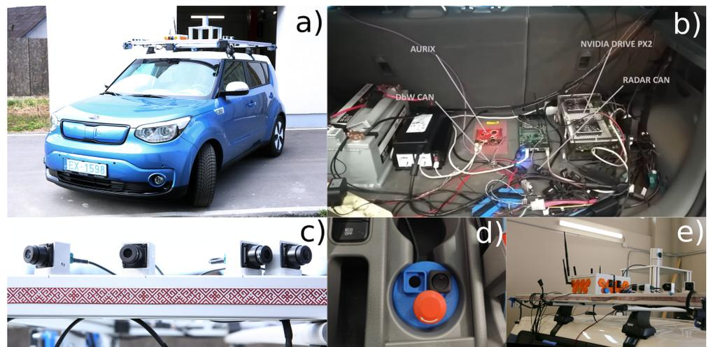
**Figure 5.** EDI perception system demonstrator. (a) EDI DbW car; (b) high-performance (NVIDIA PX2) and safety (Aurix TC3xx) controllers; (c) SEKONIX SD3323 camera mounting; (d) emergency button for exiting automatic mode; (e) EDI V2X system.
