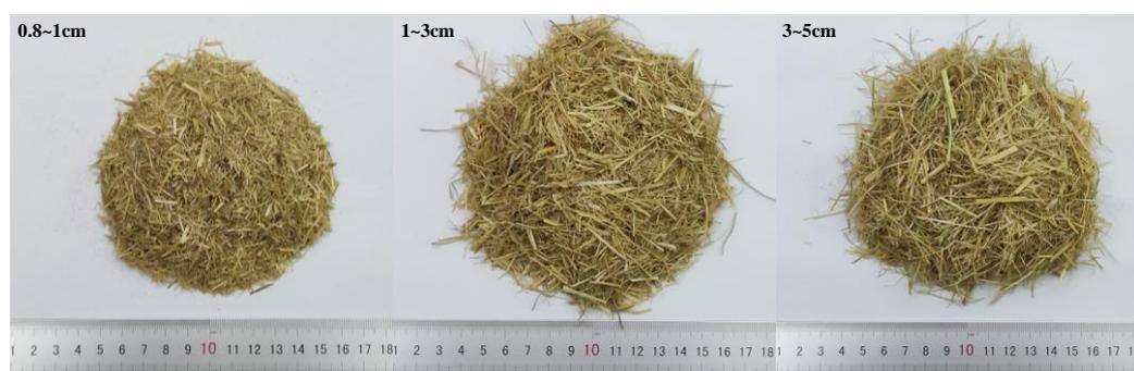
**Figure 2.** The morphology of RS fibers.
