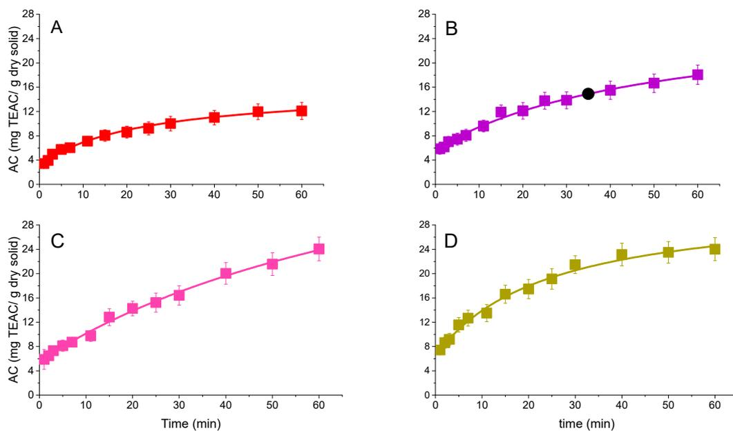
**Figure 4.** Kinetic analysis of the antioxidant activity as measured by the DPPH method during the extraction processes of AP employing a 70%/30% *v/v* ethanol/water mixture at several temperature values: (A) 25 °C, (B) 50 °C, (C) 70 °C, and (D) 90 °C. The lines show the fitting of a one-term second-order kinetic model (Equation (1)).
