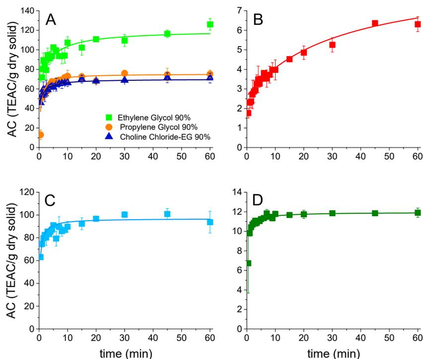
**Figure 10.** Antioxidant activity (DPPH) results, and their kinetic analysis, obtained during the extraction processes applied to GP using several solvents: (A) glycols at 70 °C; (B) acetone at 25 °C, (C) acetone 80%: water 20% at 25 °C, and (D) water at 25 °C. The lines show the second-order kinetic model (Equation (1)) fitting to data.
