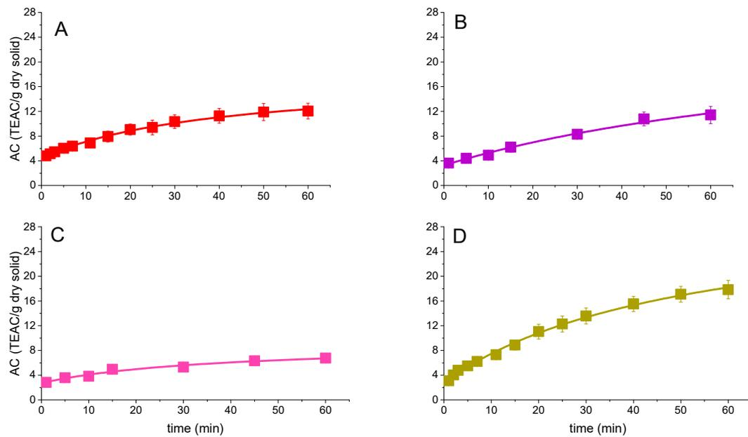
**Figure 5.** Kinetic analysis of the extraction processes of AP employing (A) acetone at 25 °C, (B) acetone/water 80%/20% *v/v* at 25 °C, (C) water at 25 °C, and (D) ethanol 96% at 70 °C: antioxidant activity as obtained by DPPH method. Kinetic model fitting is presented in lines.
