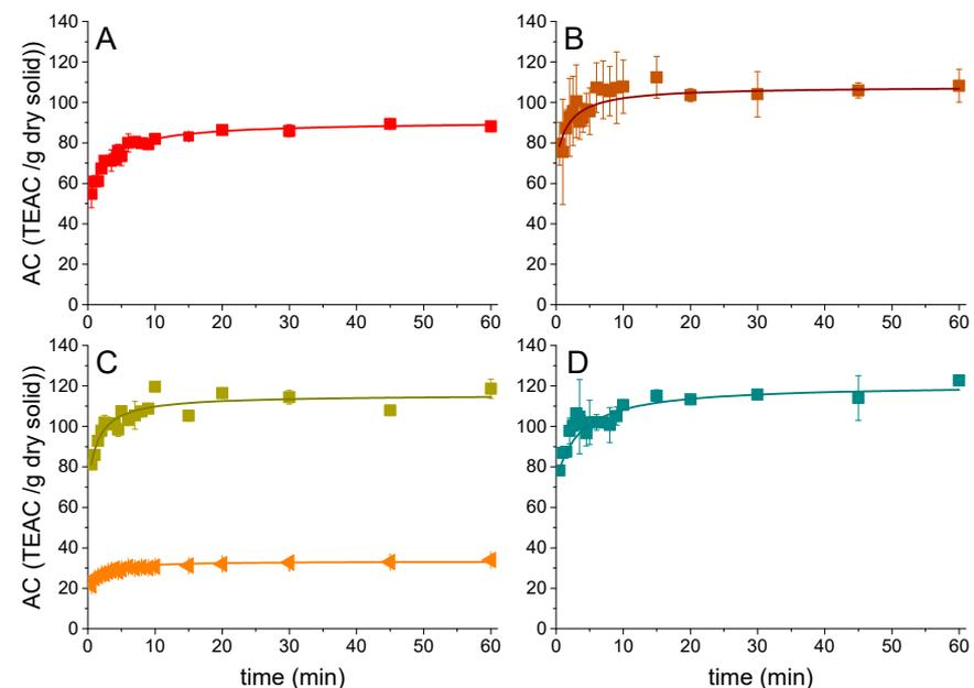
**Figure 9.** Antioxidant activity by DPPH method in points (data) and fit of the second-order kinetic model in lines. Results from grape pomace (GP) with a hydroalcoholic solution (ethanol/water 70%/30% *v/v*) at several temperatures: (A) 25 °C, (B) 50 °C, (C) 70 °C (green line and points: ethanol 70%; orange line and points: ethanol 96%), and (D) 90 °C.
