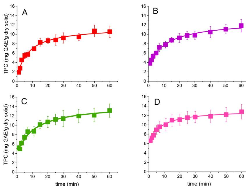
**Figure 1.** Results of total phenolic content (TPC) during extraction processes using AP and ethanol/water 70/30 (% *v/v*) at different temperatures: (A) 25 °C, (B) 50 °C, (C) 70 °C, and (D) 90 °C. Data were obtained by the Folin–Ciocalteu method. Kinetic analysis corresponding to the second-order kinetic model is displayed as lines.
