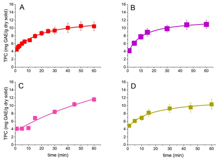
**Figure 2.** Kinetic analysis of the extraction processes of AP employing (A) acetone at 25 °C, (B) acetone 80% at 25 °C, (C) water at 25 °C, and (D) ethanol 96% (*v/v*) at 70 °C obtained by the Folin–Ciocalteu method. Fitting lines correspond to the second-order kinetic model shown in Equation (1).
