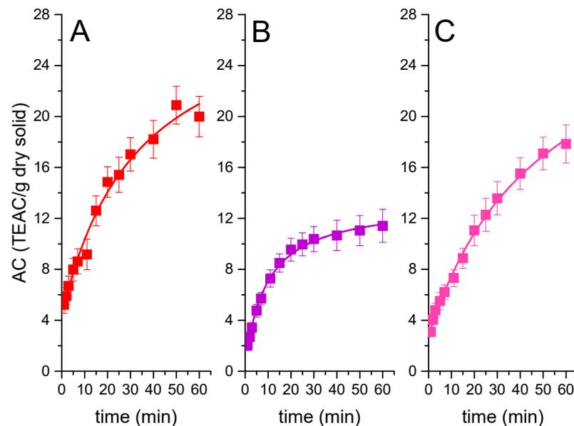
**Figure 6.** Kinetic analysis of the extraction processes of AP with glycols and a glycol-based DES at 70 °C. (A) ethylene glycol 90%, (B) propylene glycol 90%, and (C) ChCl:Gly 90%. The kinetic model fitting is presented in lines.
