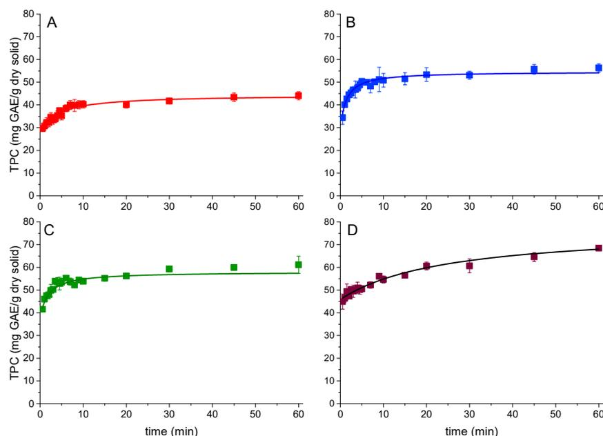
**Figure 7.** Kinetic analysis of the extraction process from grape pomace (GP) with a hydroalcoholic solution (ethanol/water 70%/30% *v/v*) at several temperatures: (A) 25 °C, (B) 50 °C, (C) 70 °C, and (D) 90 °C. Data, in points, reflects the total phenolic content (TPC) obtained by the Folin–Ciocalteu method. The lines indicate the fitting of the second-order kinetic model presented in Equation (1).
