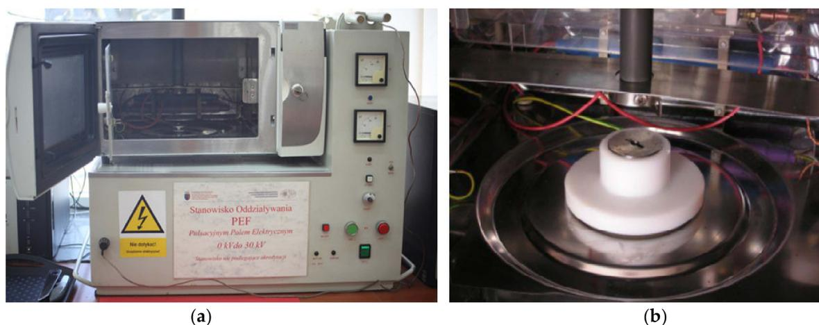
**Figure 1.** Ertec Su-1 test stand: (a) discharge chamber; (b) stationary sterilization cell.
