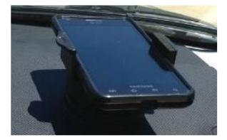
Figure 6. Mounting of the smartphone on the vehicle dashboard.
