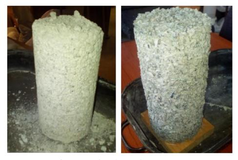
Figure 5. Specimens for CTT: GM 0/22 (left); GM 0/32 (right).
