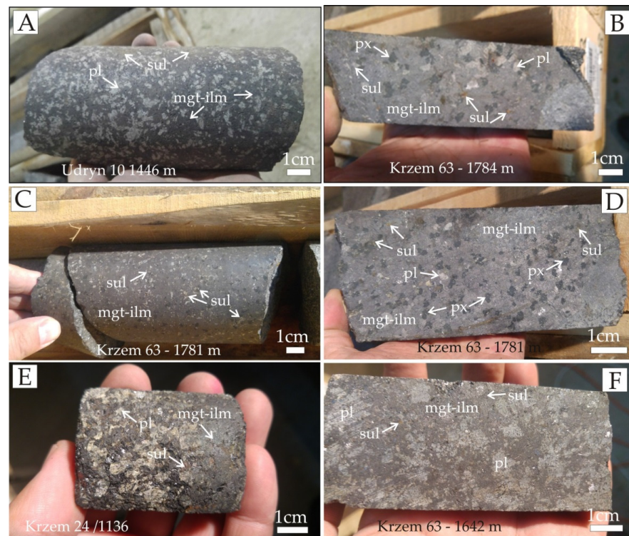
Figure 6. Typical massive and semi-massive magnetite-ilmenite (mgt-ilm) ores hosted by anorthosite or norite from the Udryn (A) and Krzemianka (B–F) deposits. Note: Krzem 63–Krzemianka 63 borehole, 1784 m—an approximate depth of sampling. Abbreviations: mgt-ilm—magnetite-ilmenite; pl—plagioclase; px—pyroxene; sul—sulphides.
