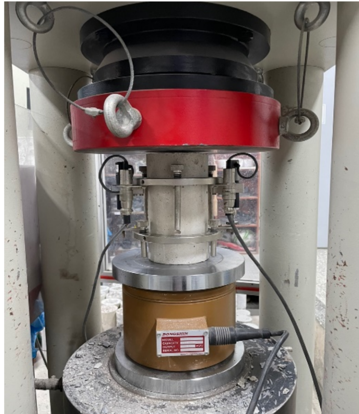
Figure 3. Compressive strength and elastic modulus test.
