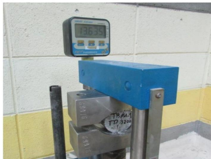
Figure 1. Failure of a sample under a BTS test [3].
