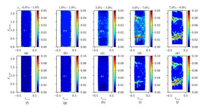
**Figure 12.** The evolution of the standard deviation fields of *divergence div U*: ( $\mathbf{a}$ - $\mathbf{e}$ ) the standard deviation fields of *div U* at axial strains of 0.0–1.0%, 1.0–3.0%, 3.0–5.0%, 5.0–7.0%, and 7.0–9.0%, respectively, with varying range colormaps; ( $\mathbf{f}$ - $\mathbf{j}$ ) the standard deviation fields of *div U* at axial strains of 0.0–1.0%, 1.0–3.0%, 3.0–5.0%, 5.0–7.0%, and 7.0–9.0%, respectively, with consistent range colormaps.
