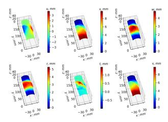
**Figure 3.** Incremental displacement fields of test 092903b between an axial strain of 3.0% and 9.0% (post-peak of the stress–strain curve). The first row from left to right are displacements along horizontal (u), vertical (v), and out-of-plane (w) directions. The second row describes the same displacement field, but decomposed into radial (r), tangential (t), and axial (v) directions in cylindrical coordinates.
