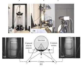
**Figure 2.** The experimental setup: (a) triaxial compression system; (b) the 3D-DIC system; (c) a schematic illustration of a common section captured by two camera systems.
