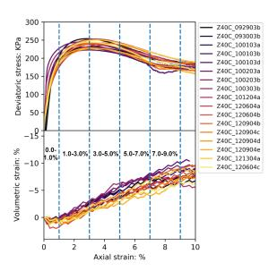
**Figure 1.** The triaxial stress–strain and volumetric–axial strain curves of 17 tests. Dashed intervals indicate the temporal increments of kinematic analysis.
