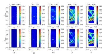
**Figure 10.** The evolution of the standard deviation fields of the *gradient* along the  $\hat{y}$  axis  $F_{33}$ : (**a–e**) the mean fields of  $F_{33}$  at axial strains of 0.0–1.0%, 1.0–3.0%, 3.0–5.0%, 5.0–7.0%, and 7.0–9.0%, respectively, with varying range colormaps; (**f–j**) the mean fields of  $F_{33}$  at axial strains of 0.0–1.0%, 1.0–3.0%, 3.0–5.0%, 5.0–7.0%, and 7.0–9.0%, respectively, with consistent range colormaps.
