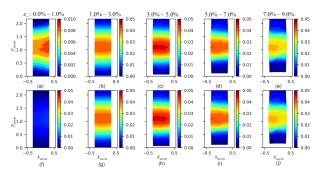
**Figure 7.** The evolution of the mean fields of gradient along the  $\hat{\rho}$  axis  $F_{11}$ : (**a–e**) mean fields of  $F_{11}$  at axial strains of 0.0–1.0%, 1.0–3.0%, 3.0–5.0%, 5.0–7.0%, and 7.0–9.0%, respectively, with varying range colormaps; (**f–j**) mean fields of  $F_{11}$  at axial strains of 0.0–1.0%, 1.0–3.0%, 3.0–5.0%, 5.0–7.0%, and 7.0–9.0%, respectively, with consistent range colormaps.
