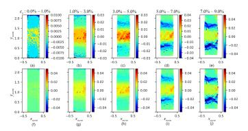
**Figure 11.** The evolution of the mean fields of *divergence div U*: ( $\mathbf{a}$ - $\mathbf{e}$ ) the mean fields of *div U* at axial strains of 0.0–1.0%, 1.0–3.0%, 3.0–5.0%, 5.0–7.0%, and 7.0–9.0%, respectively, with varying range colormaps; ( $\mathbf{f}$ - $\mathbf{j}$ ) the mean fields of *div U* at axial strains of 0.0–1.0%, 1.0–3.0%, 3.0–5.0%, 5.0–7.0%, and 7.0–9.0%, respectively, with consistent range colormaps.
