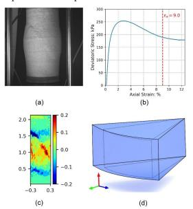
**Figure 5.** An example of a *divergence* field of test 092903b at axial strains between  $\varepsilon_a = 0.0\%$  and  $\varepsilon_a = 9.0\%$ : (a) specimen image at an axial strain of  $\varepsilon_a = 9.0\%$ ; (b) stress–strain curve of the test and strain moment of  $\varepsilon_a = 9.0\%$ ; (c) *divergence* field calculated between  $\varepsilon_a = 0.0\%$  and  $\varepsilon_a = 9.0\%$ ; (d) schematic illustration of the positive *divergence* field in cylindrical coordinates.
