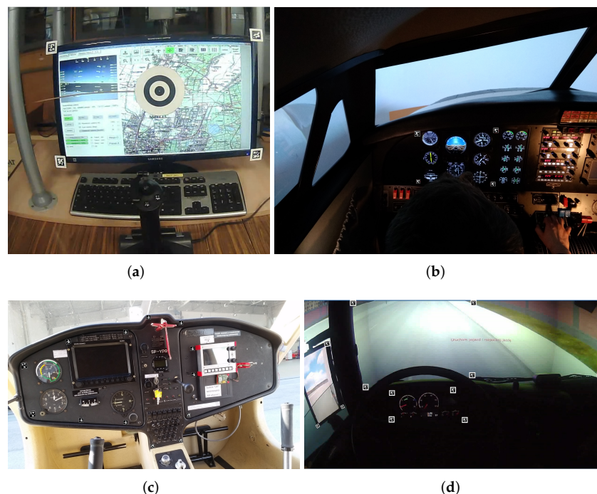
Figure 2. Observer attention recording and analysis stand (a) RPAS, (b) GA simulator (cockpit view), (c) flying lab (cockpit view), (d) truck simulator (cockpit view).
