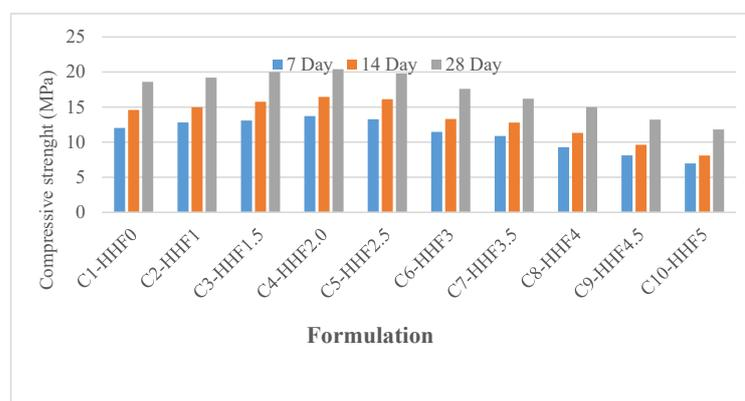
Figure 1. Compressive strength of concrete human hair fiber.
