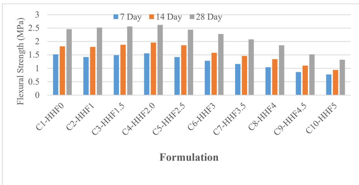
Figure 4. Flexural strength of concrete human hair fiber.
