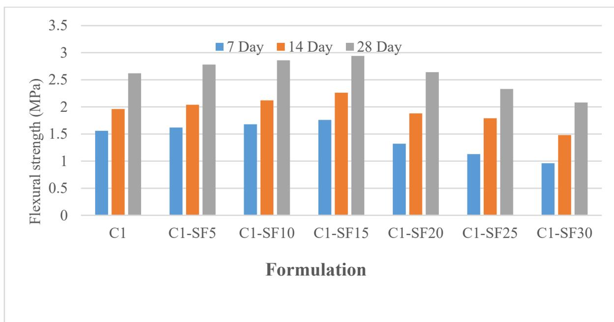
**Figure 5.** Flexural strength of concrete human hair fiber with silica fume.
