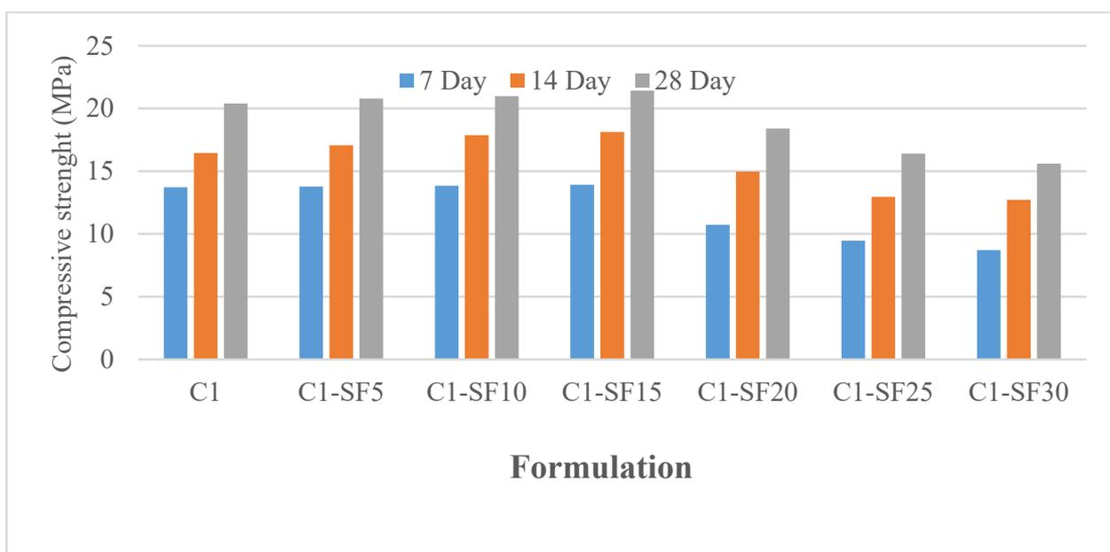
**Figure 2.** Compressive strength of concrete human hair fiber with Silica fume.
