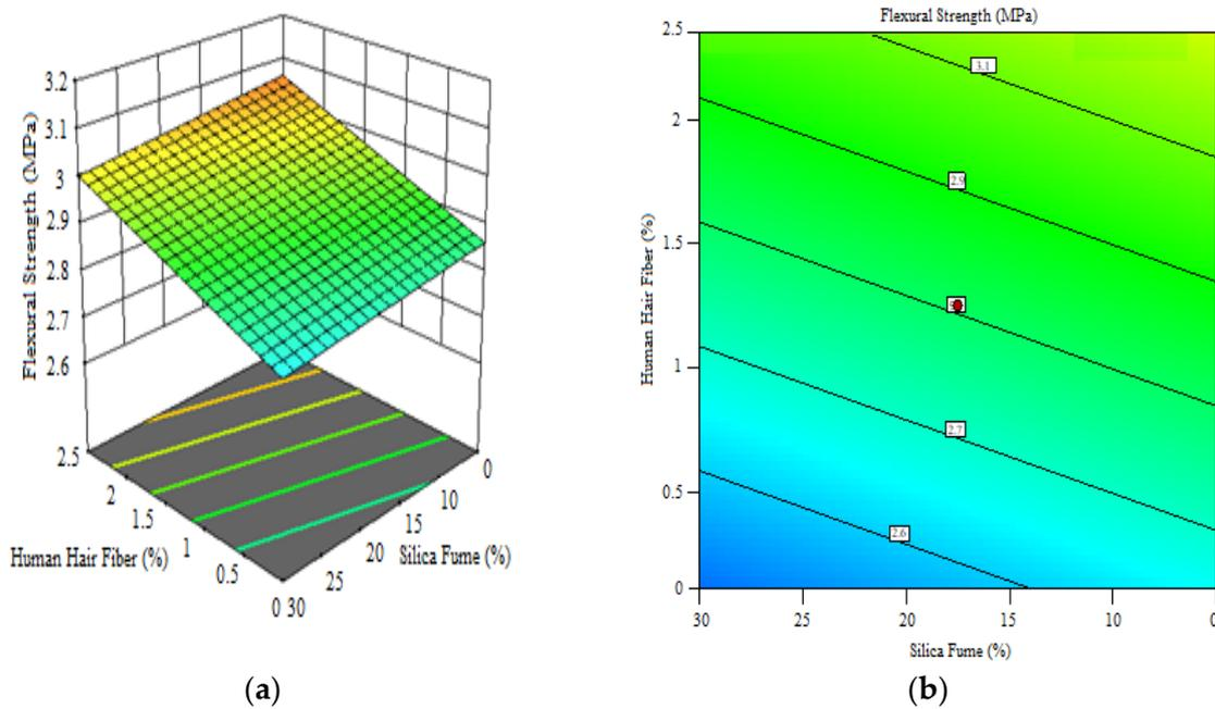
Figure 6. (a) 3D surface diagram for flexural strength; (b) 2D contour for flexural strength.
