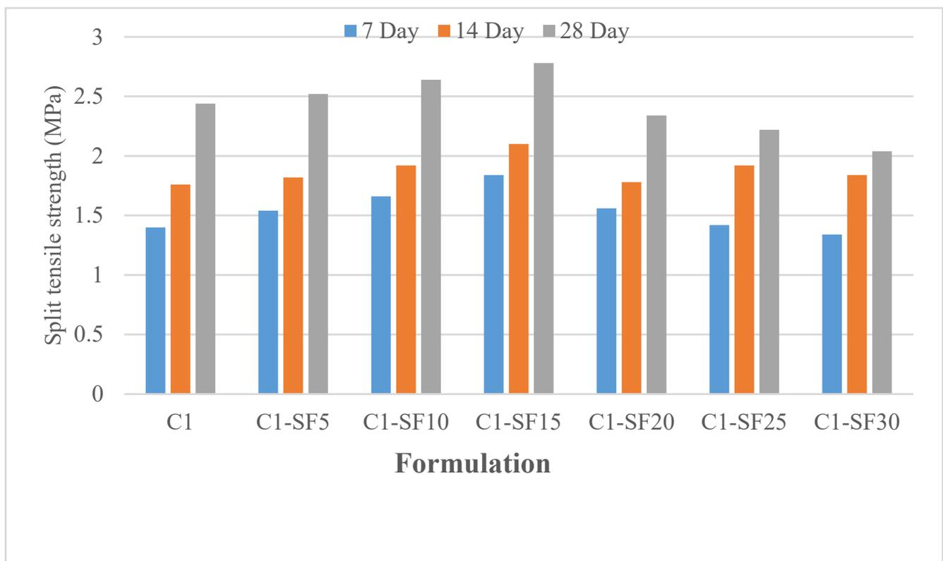
**Figure 8.** Split tensile strength of concrete human hair fiber with silica fume.
