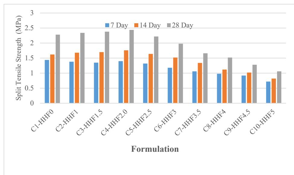
Figure 7. Split tensile strength of concrete human hair fiber.
