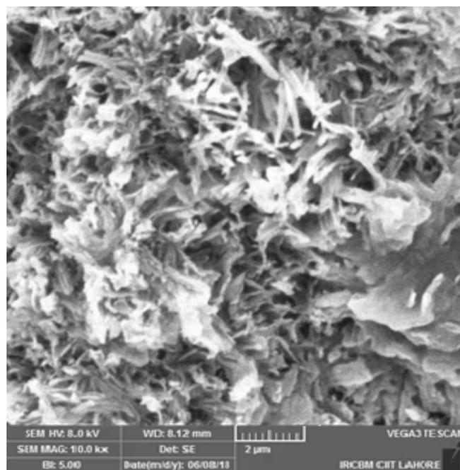
Figure 10. SEM of human hair fiber concrete.
