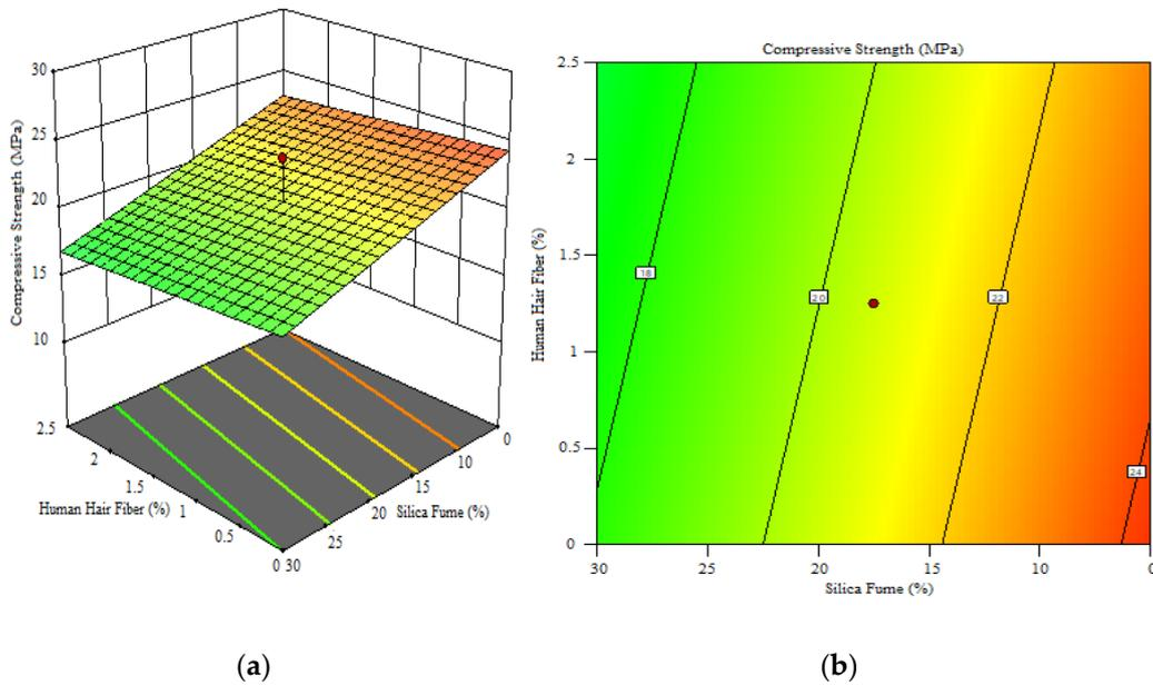
Figure 3. (a) 3D surface diagram for compressive strength; (b) 2D contour for compressive strength.
