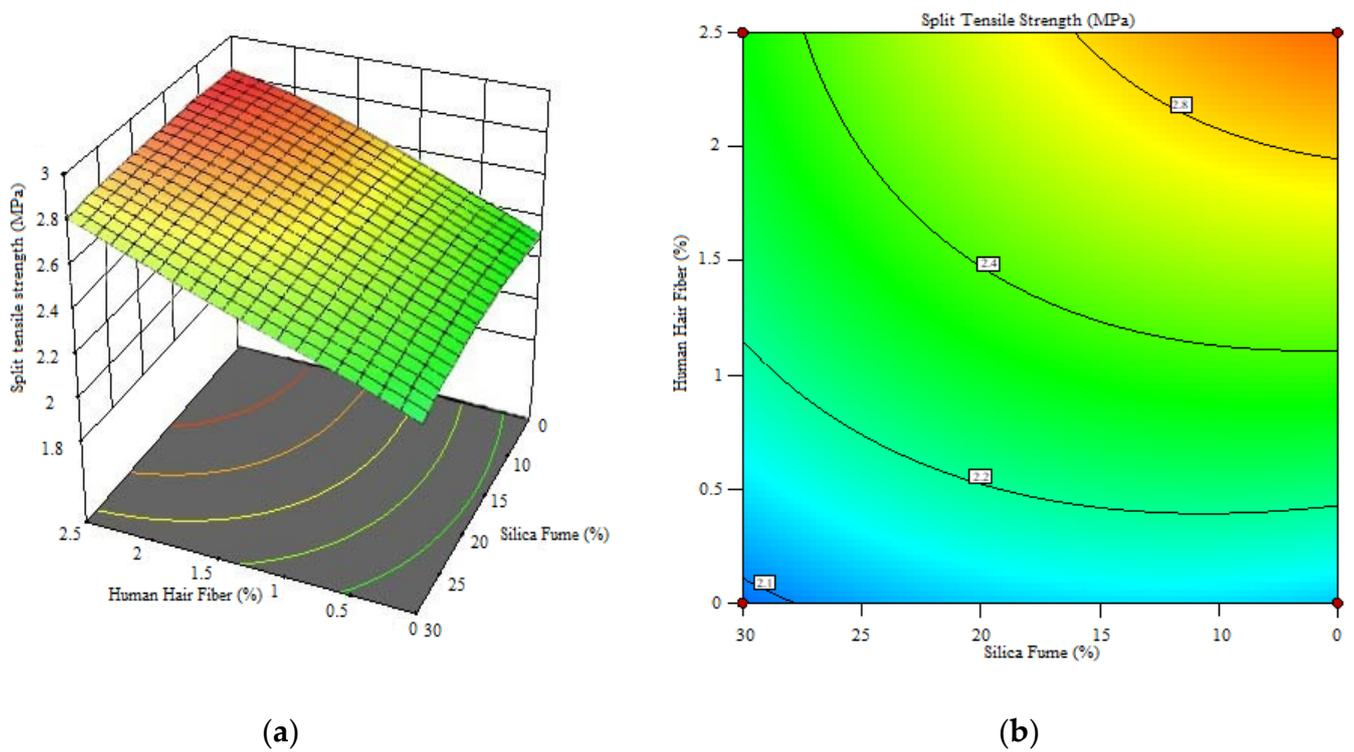
Figure 9. (a) 3D surface diagram for split tensile strength; (b) 2D contour for split tensile strength.
