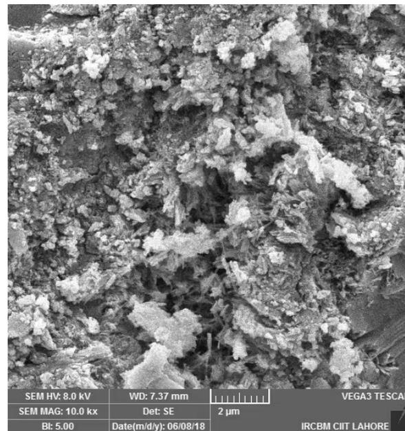
**Figure 11.** SEM of human hair fiber concrete incorporation silica fume.
