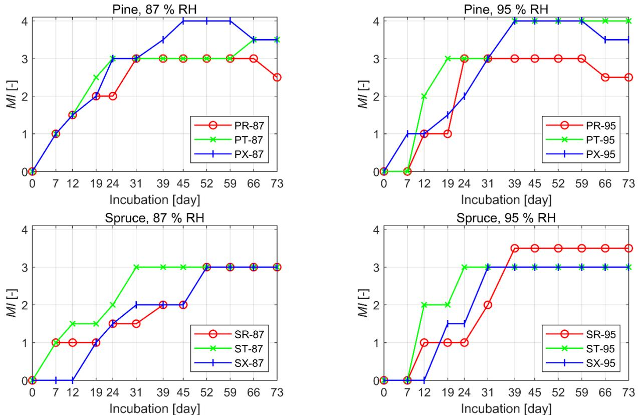
Figure 3. Mold index  $MI$  (defined according to Table 2) over time for all wood specimens tested. The mold growth curves are presented as the average for each subset of specimens.
