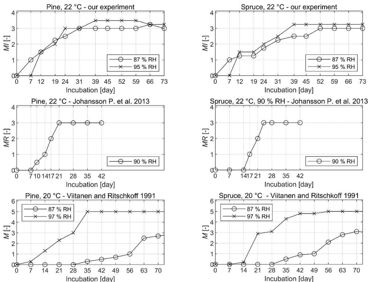
**Figure 4.** Comparison of experimental mold growth curves (our experiment—mean mold growth curves calculated from specimens with radial and tangential surfaces, data of Johansson et al. 2013 [12], data of Viitanen and Ritschkoff 1991 [19]. The time for the first microscopic signs of molds corresponds to  $MR = 1$  and  $M = 1$ . The time for the first macroscopic signs of molds corresponds to  $MR = 3$  and  $M = 3$ .
