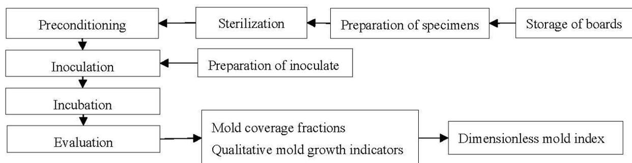
**Figure 1.** Scheme of the mold growth experiment.
