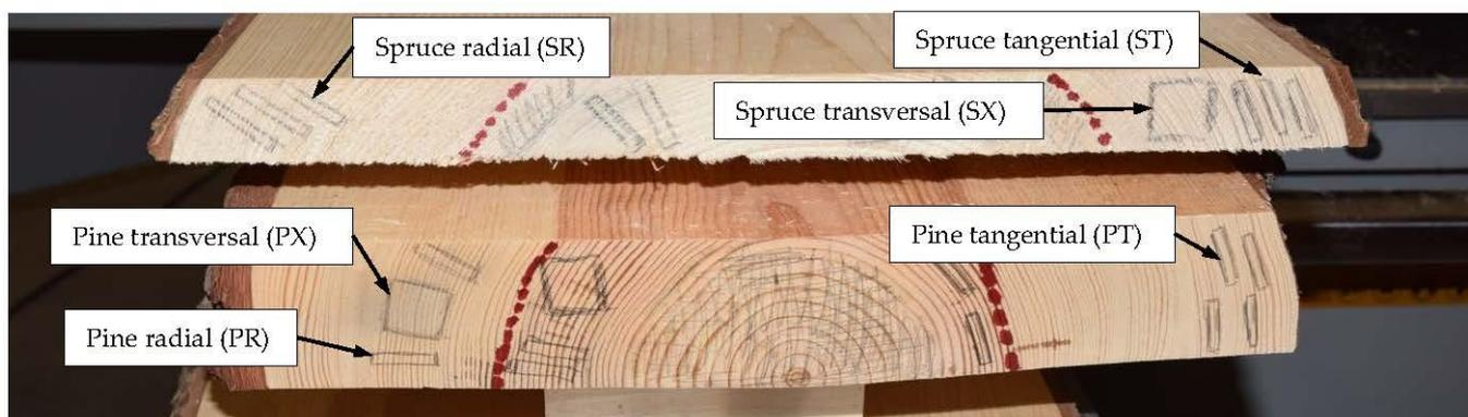
**Figure 2.** Boards used for the preparation of wood specimens. Spruce board is located on the top, pine board on the bottom. Red dashed lines separate heartwood and sapwood.
