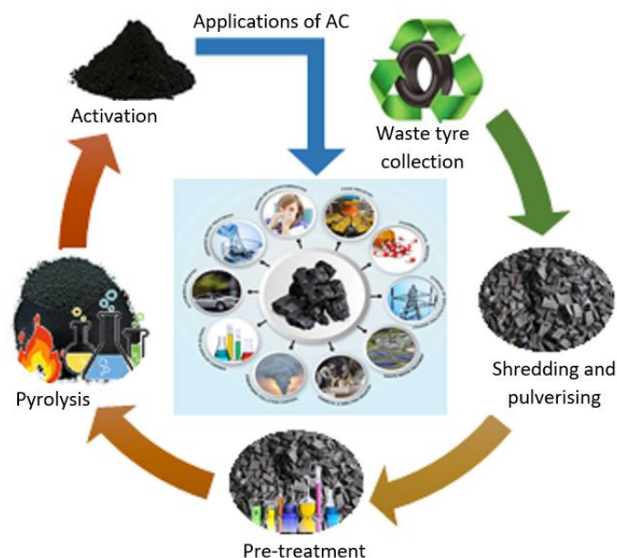
Figure 1. Steps involved in the production of activated carbon from waste tyres.
