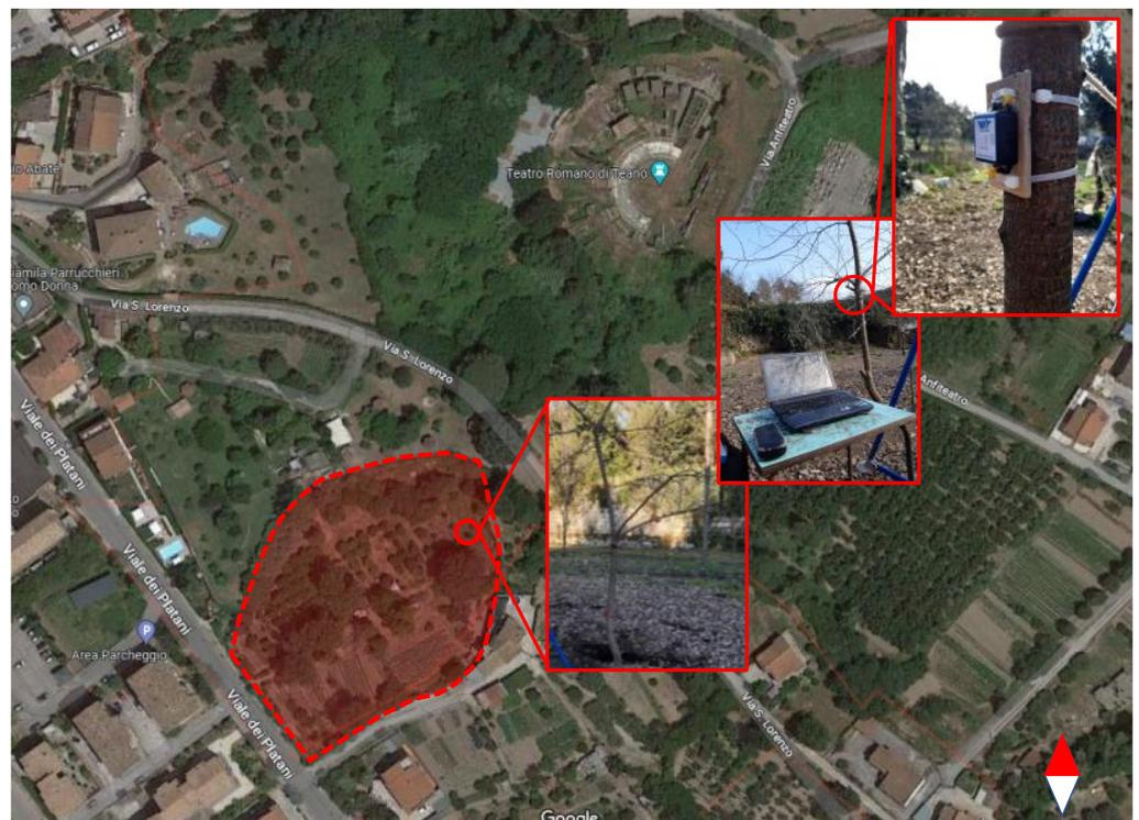
**Figure 2.** Overview of the site, the tree, and measurement setup (accelerometer). [Google Earth].
