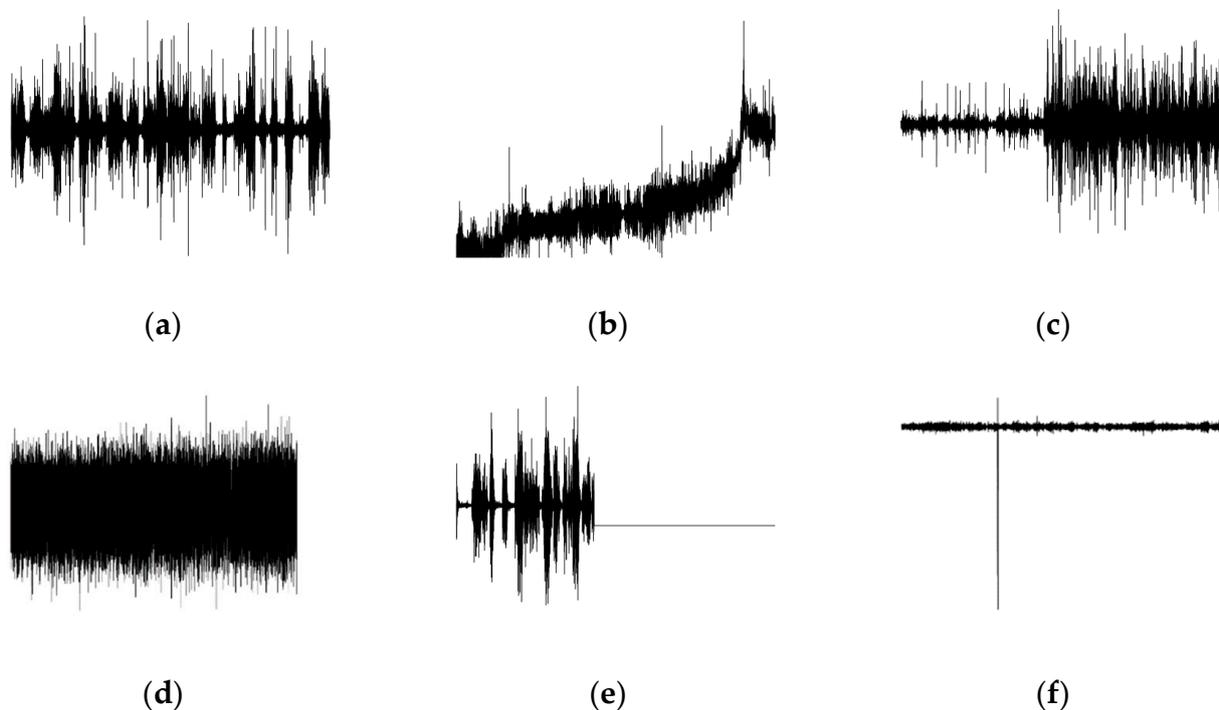
**Figure 1.** Schematic diagram of data characteristics of each category. (a) normal. (b) drift. (c) local gain. (d) noise. (e) missing. (f) outlier.
