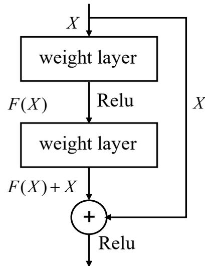
**Figure 3.** Residual block construction.
