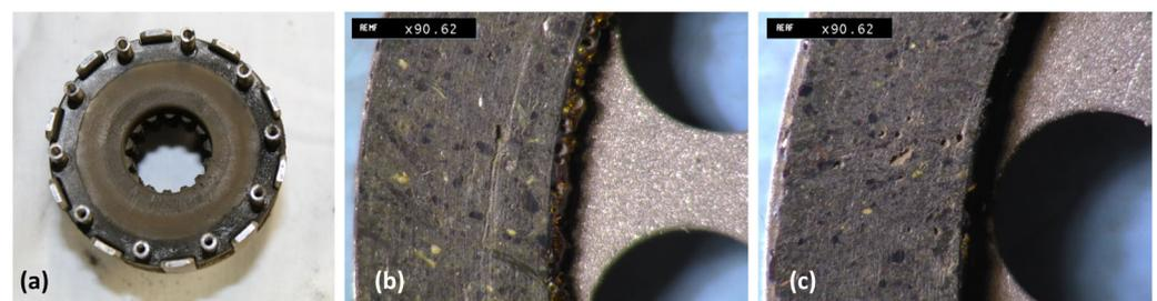
**Figure 22.** Worn components: (a) solenoid; (b) rotor 1; (c) rotor 2.
