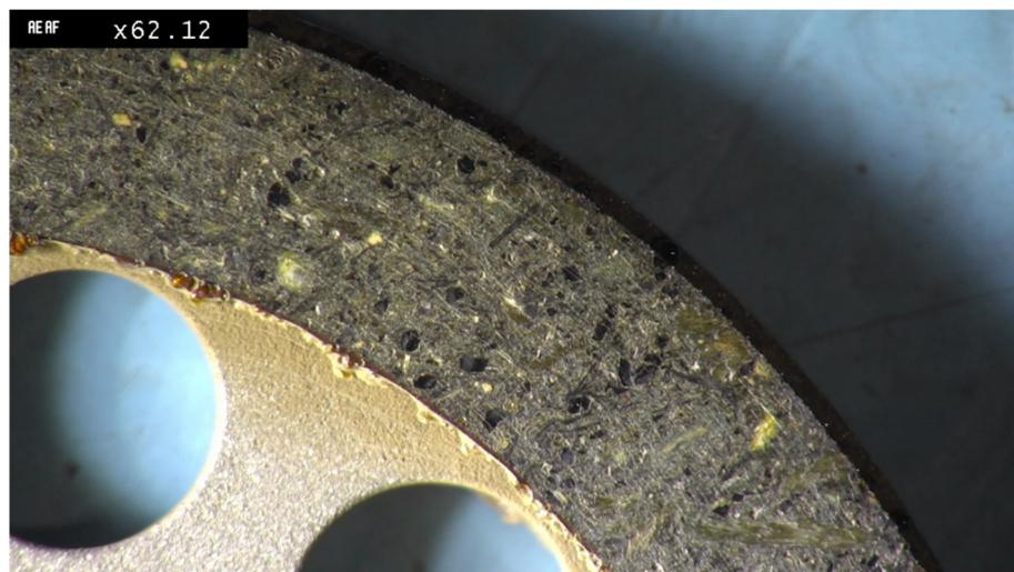
**Figure 16.** Rotor disk with NAO as friction material.
