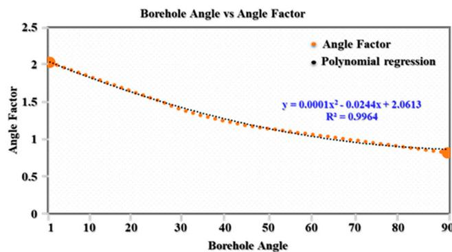
Figure 6. The interpolation of  $AF$  based on the borehole angle.
