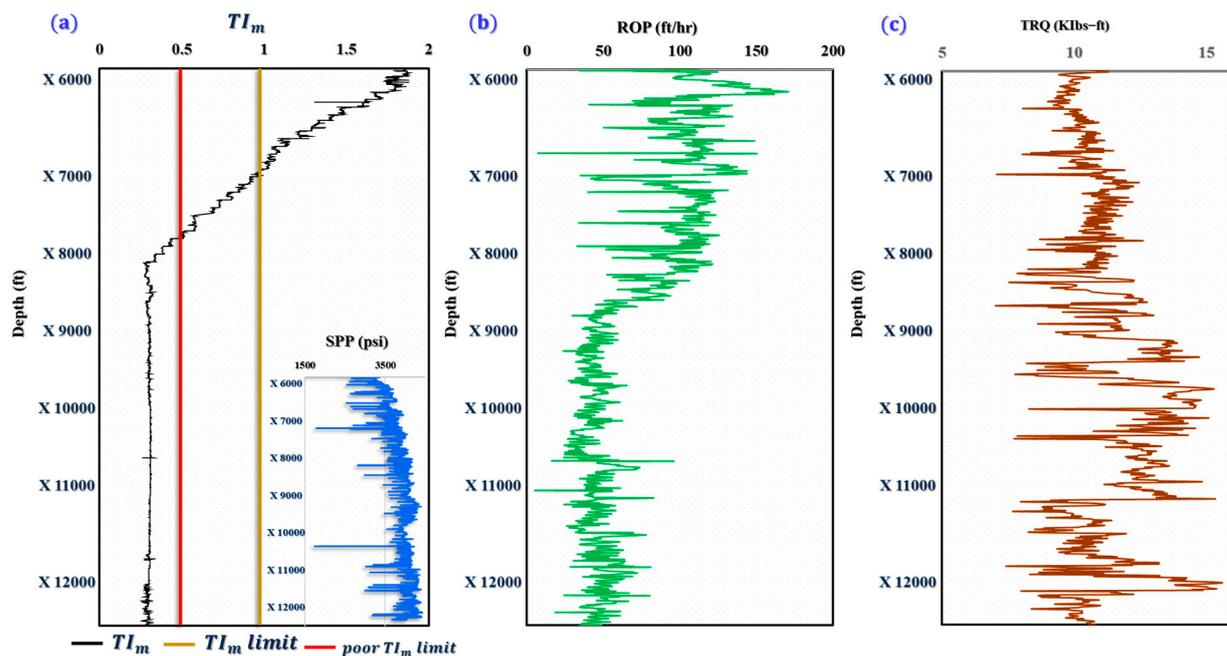
**Figure 13.** Application of  $TI_m$  in Well C in the case of a stuck pipe: (a) Well-C with poor borehole cleaning, (b) ROP, and (c) TRQ.
