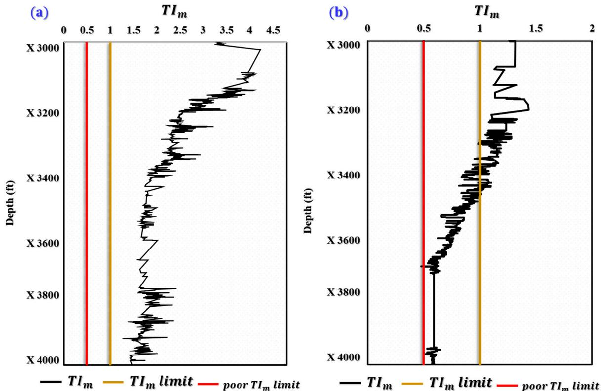
**Figure 11.** Application of  $TI_m$  in offshore Well-A with proper borehole cleaning (a) and Well-B with poor borehole cleaning (b).
