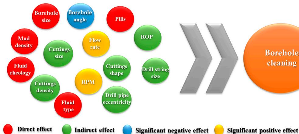
**Figure 2.** Parameters and their effect on borehole cleaning.
