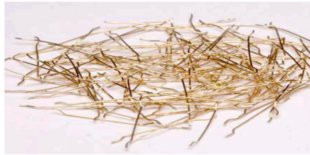
Figure 6. Fiber material used in the UHPFRC matrix.
