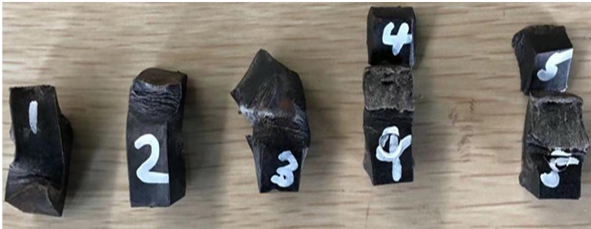
Figure 9. Specimens collapsed in the compression test.
