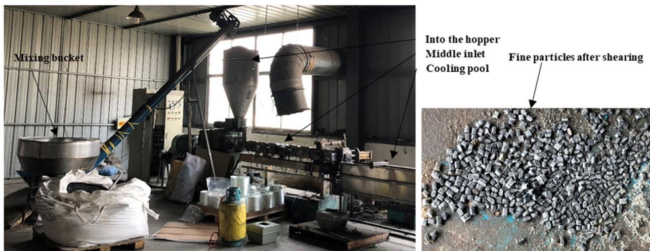
**Figure 4.** Twin screw extruder and granulation.
