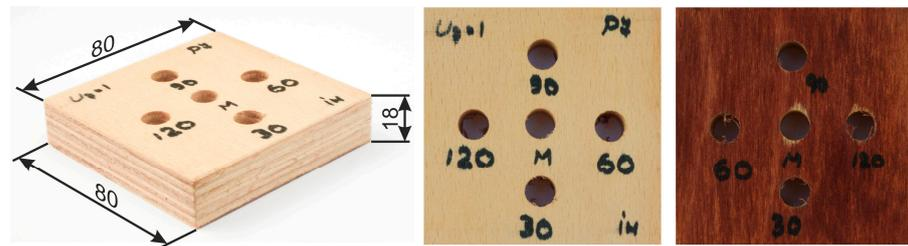
Figure 2. The plywood samples used during drilling experiments.
