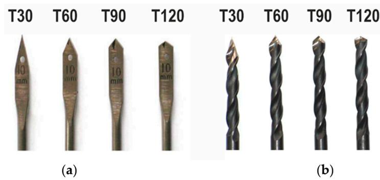
Figure 1. The drill bits used in the experiments: (a) flat drills; (b) helical drills.
