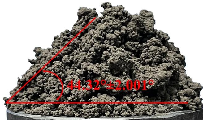
**Figure 5.** Soil AoR test.
