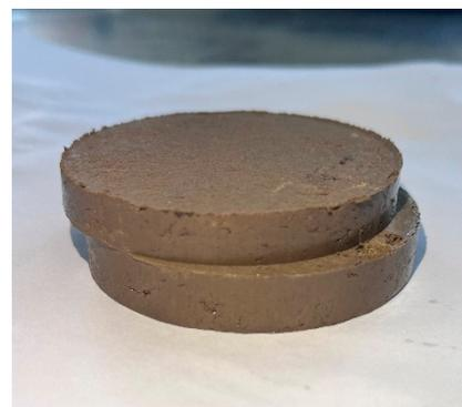
**(b)** Soil samples after direct shear.
