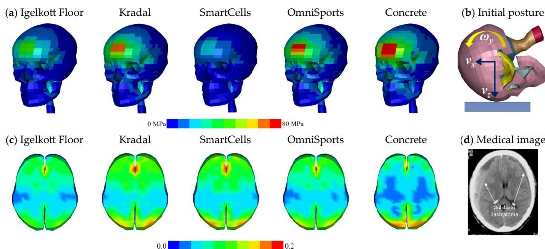
**Figure 7.** (a) Comparison of peak von Mises stresses (MPa) on the cortical bone against four EAFs and concrete ground of Case 3. (b) Accident reconstruction of head impact initial posture on forward falling. (c) Comparison of the peak 1st principal strain on the brain tissue of Case 3. (d) the medical image of Case 3, which is from the research [52]. Copyright (CC BY-NC-ND 3.0 IE).
