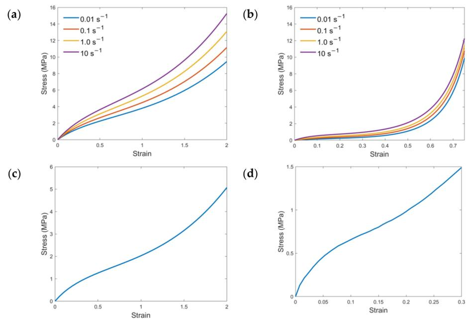
**Figure A1.** The stress–strain curves of four EAF specimens used in LS-DYNA, (a) tension tests of Igelkott Floor, (b) compression tests of Kradal, (c) tension tests of SmartCells, (d) compression tests of OmniSports, respectively.
