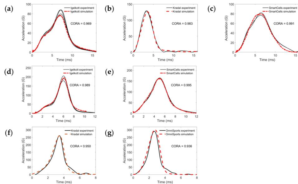
**Figure 5.** The acceleration–time curves for HIII drop tests and hemispheric drop tests, with related overall CORA score, (a) Igelkott Floor HIII 60 cm; (b) Kradal HIII 60 cm; (c) SmartCells HIII 60 cm; (d) Igelkott Floor HIII 100 cm; (e) SmartCells HIII 100 cm; (f) Kradal hemispheric 60 cm; (g) OmniSports hemispheric 60 cm.
