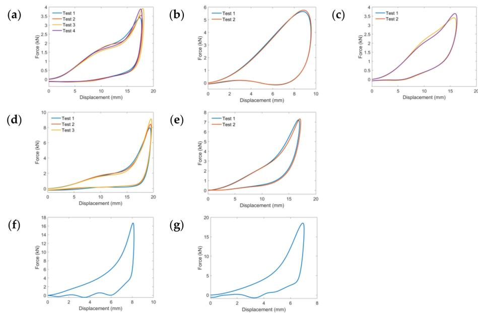
**Figure A3.** The force–displacement curves for HIII drop tests and hemispheric drop tests, (a) Igelkott Floor HIII 60 cm; (b) Kradal HIII 60 cm; (c) SmartCells HIII 60 cm; (d) Igelkott Floor HIII 100 cm; (e) SmartCells HIII 100 cm; (f) Kradal hemispheric 60 cm; (g) OmniSports hemispheric 60 cm.
