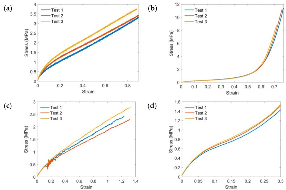
**Figure A2.** The experimental stress–strain curves of four EAF specimens from mechanical tests under the same strain rate, (a) tension tests of Igelkott Floor, (b) compression tests of Kradal, (c) tension tests of SmartCells, (d) compression tests of OmniSports, respectively.
