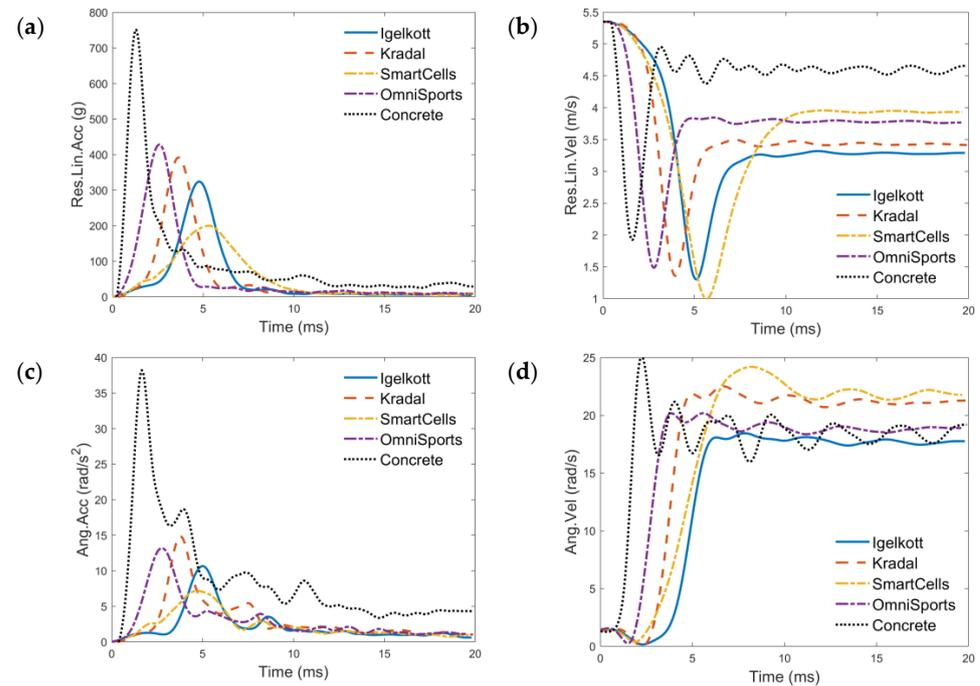
**Figure 6.** The kinematics–time curves of the head CG in fall accident reconstructions case [52] against four types of EAFs: (a) resultant linear acceleration, (b) resultant linear velocity, (c) angular acceleration, (d) angular velocity.
