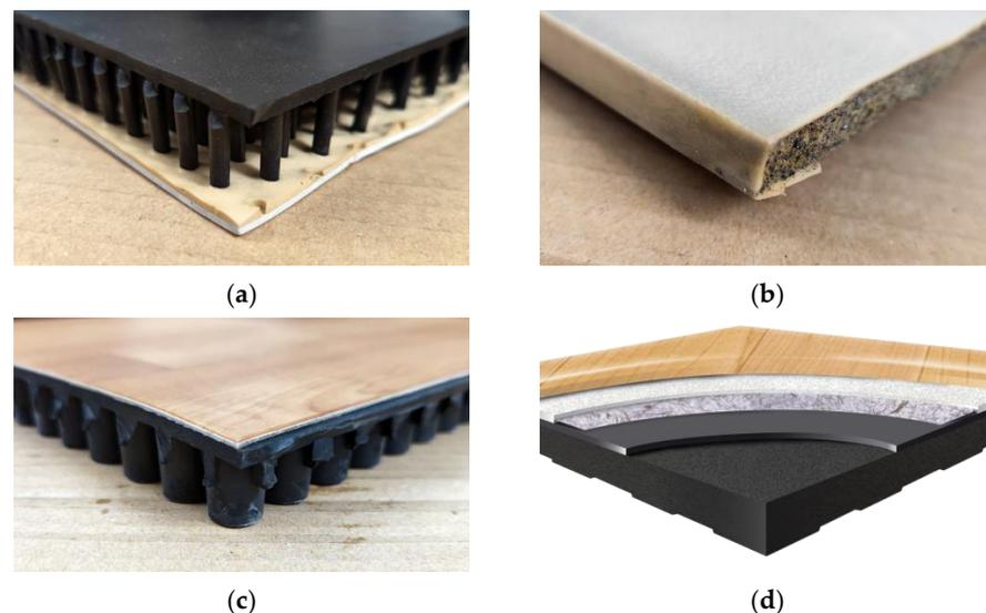
**Figure 1.** Four types of energy-absorbing flooring samples compared in this study. The image of (d) Omnisports is from its official website (<https://proffs.tarkett.se/>, accessed on 22 April 2023). (a) Igelkott Floor; (b) Kradal; (c) SmartCells; (d) Omnisports.
