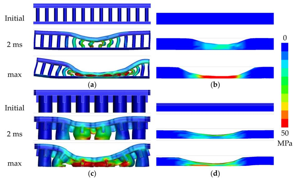
**Figure 8.** Comparison of peak von Mises stresses (MPa) of four energy-absorbing floors in the accident reconstruction case: the former is at 2 ms and the latter is at the maximum deformation state, respectively. (a) Igelkott Floor; (b) Kradal; (c) SmartCells; (d) OmniSports.
