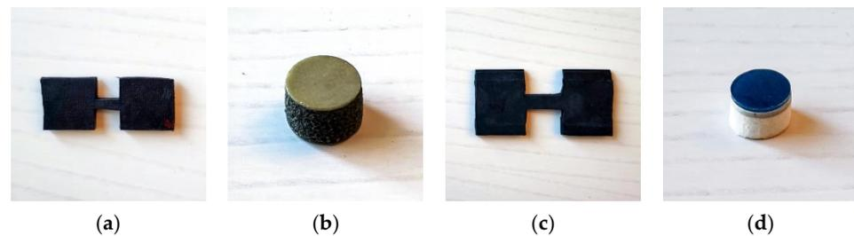
**Figure 2.** Four energy-absorbing floor specimens for the compression/tension tests. (a) Igelkott Floor; (b) Kradal; (c) SmartCells; (d) OmniSports.
