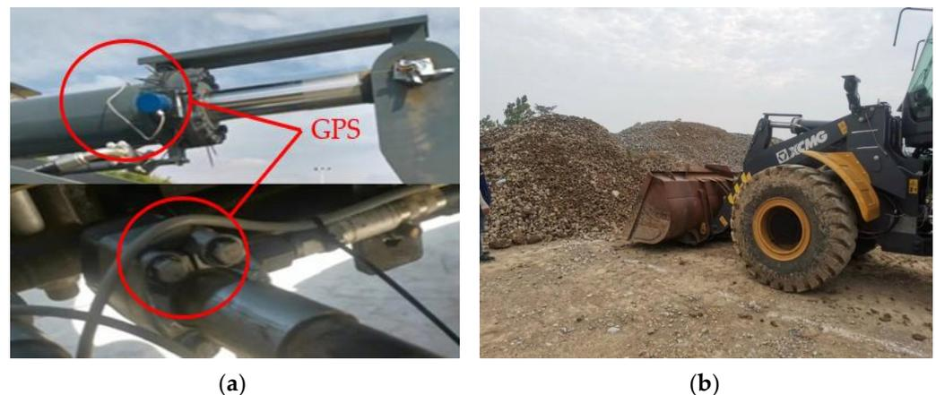
**Figure 5.** Dynamic calibration experiment: (a) GPS layout; (b) shoveling process.
