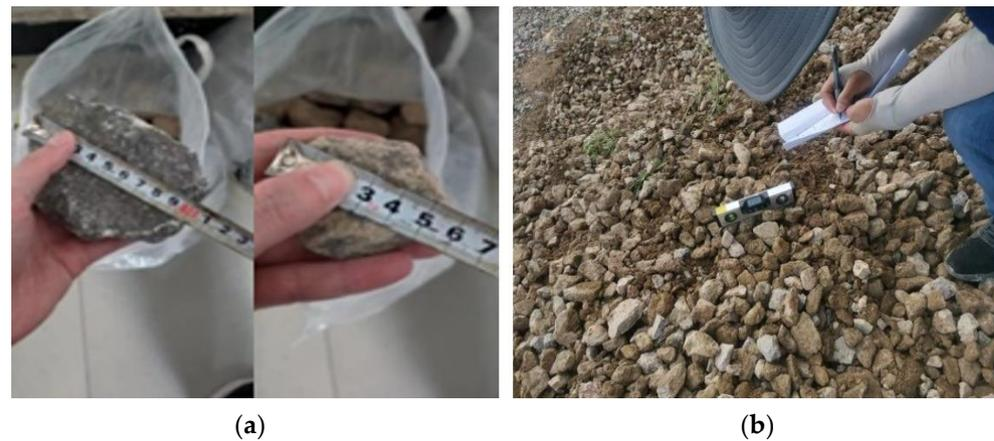
**Figure 4.** Static calibration experiment: (a) particle size measurement in ore samples; (b) repose angle measurement in ore samples.
