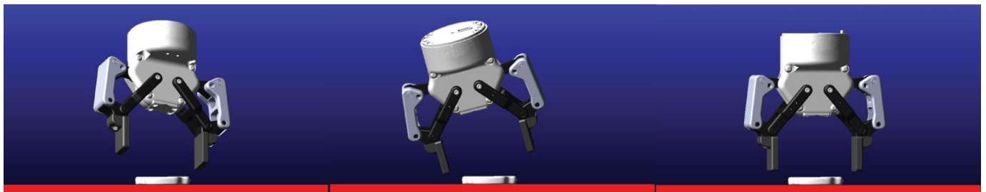
Figure 3. Model of robotic gripper and the object to be gripped in ADAMS/View with different rotation settings. Source: Own.
