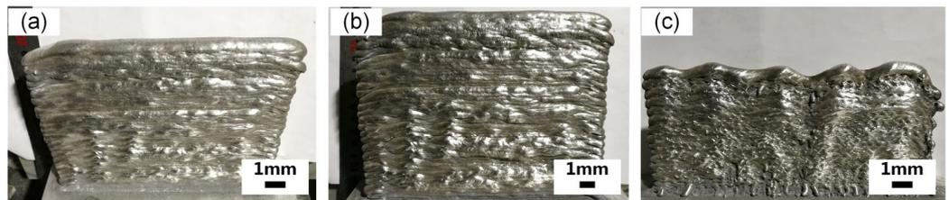
**Figure 2.** Side-wall morphology of magnesium deposited sample: (a) overview of No. 1, (b) No. 1, (c) No. 2.
