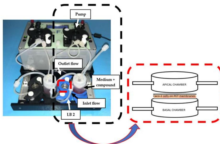
**Figure 2.** LiveFlow<sup>®</sup> bioreactor in our set-up.
