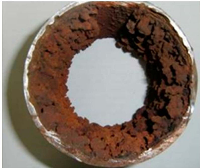
Figure 1. A fragment of steel galvanized pipe with corrosion tubercles.
