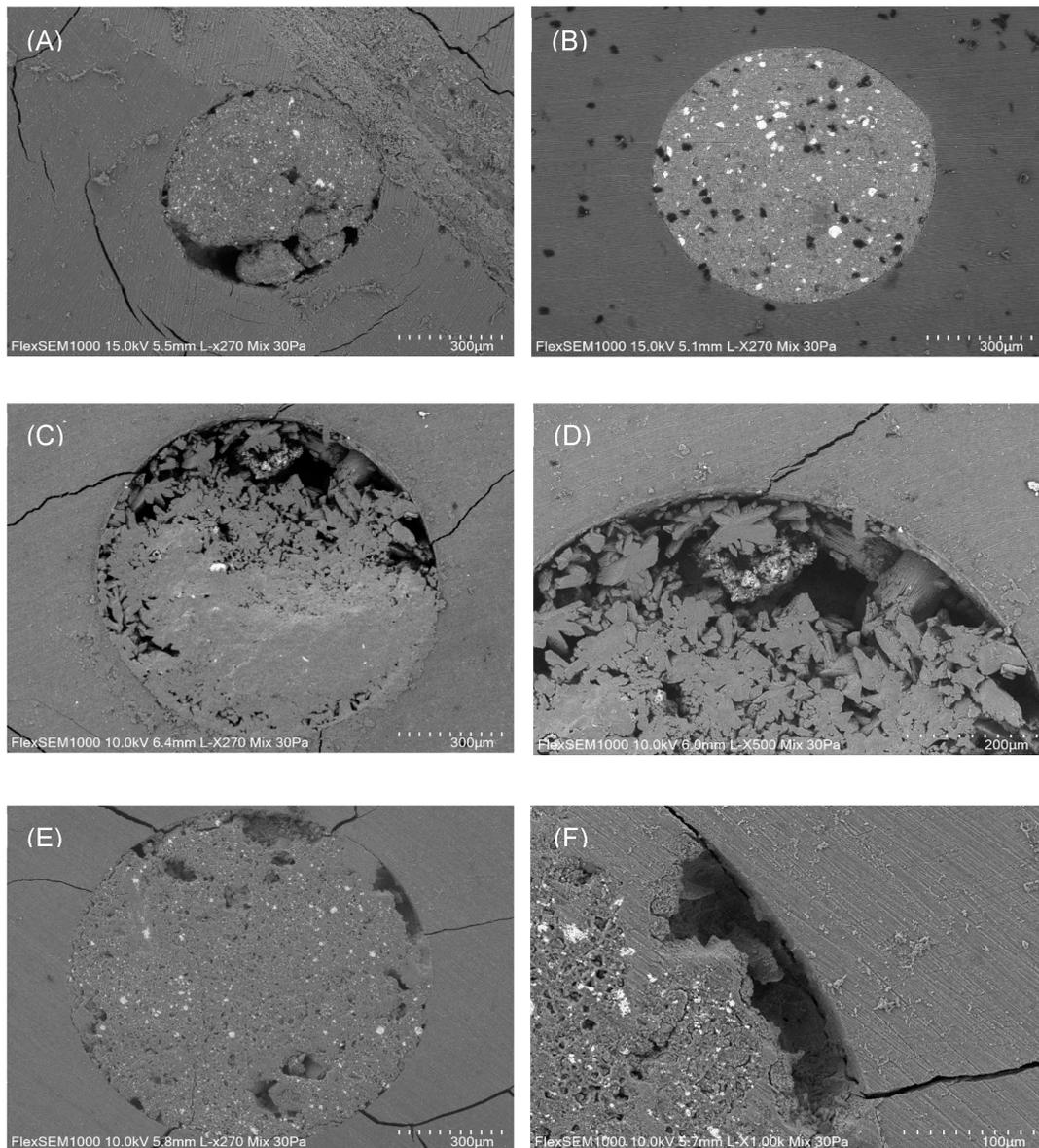
**Figure 2.** Scanning electron microscopy image. (A) White ProRoot MTA<sup>®</sup> plug in the apical region; (B) TotalFill<sup>®</sup> BC RRM Fast Set Putty<sup>™</sup> plug in the apical region (270× magnification). (C) TotalFill<sup>®</sup> BC RRM Fast Set Putty<sup>™</sup> plug in the cervical region (270×) and (D) 500×. (E): White ProRoot MTA<sup>®</sup> plug in the cervical region (270) and (F) 1000× of amplification.
