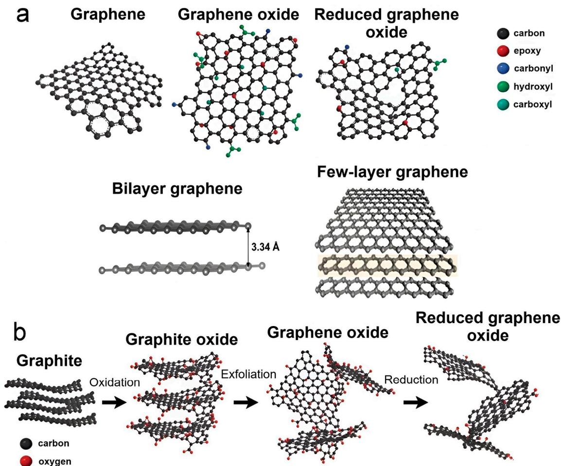
**Figure 4.** Possible types of graphene and representation of the process of obtaining reduced graphene oxide by oxidative exfoliation of graphite. (a) Types of graphene and the main oxygen-containing functional groups on its edges; (b) Scheme for obtaining reduced GO from graphite by chemical treatment.
