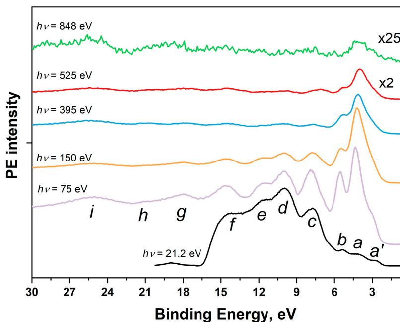
**Figure 8.** VB PE spectra of the [Ni(Salen)] complex excited by photons with energies  $h\nu$  from 21.2 eV to 848 eV. The lowercase letters  $a'$ ,  $a$ ,  $b$ ,  $c$ ,  $d$ ,  $e$ ,  $f$ ,  $g$ ,  $h$  and  $i$  denote the photoemission signals of individual sub-bands of the valence band [53].
