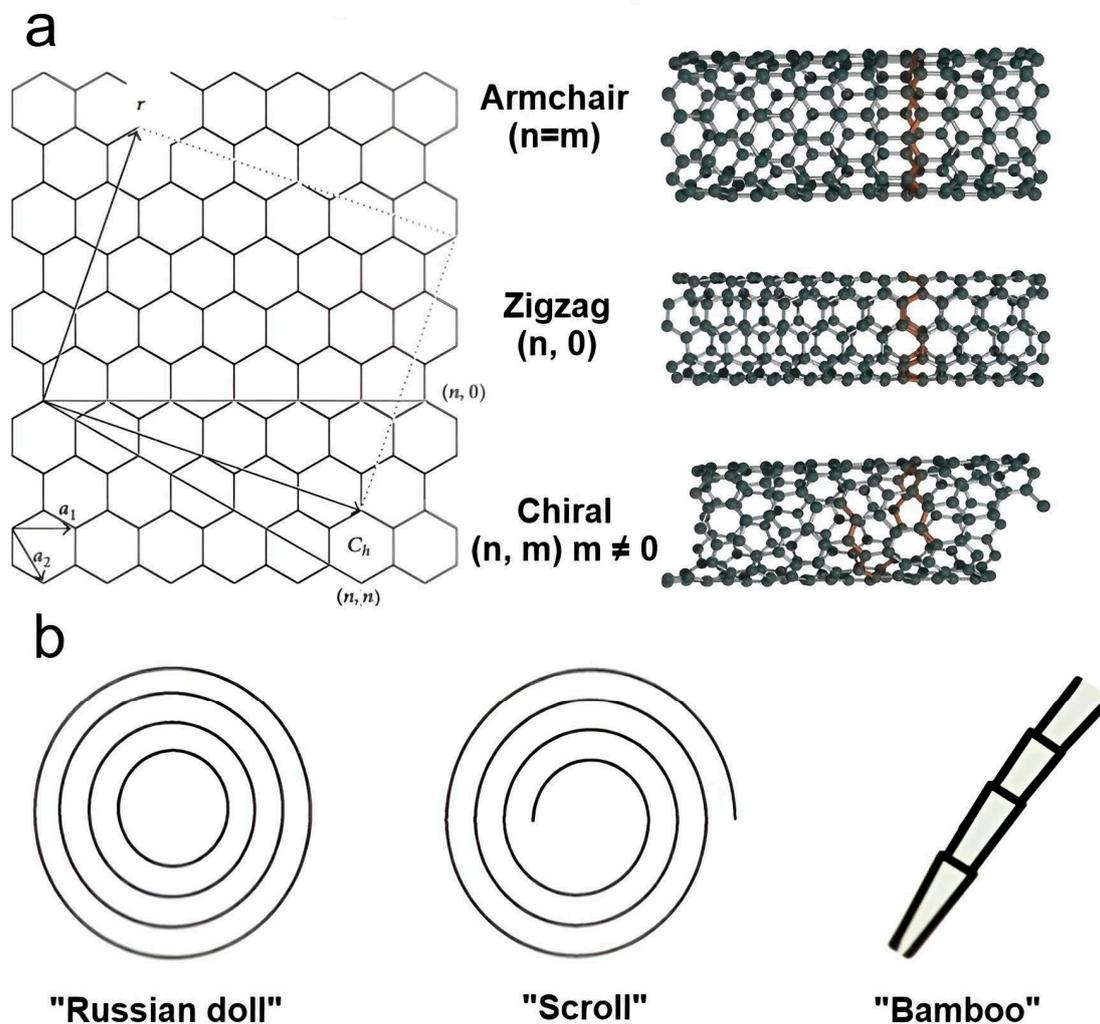
**Figure 3.** The main types of carbon nanotubes: (a) variants of SWCNTs constructed from a graphene sheet along the chiral vector  $C_h$  and (b) various forms of MWCNTs.
