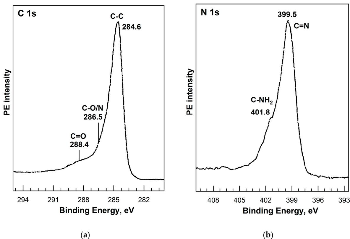
Figure 17. C 1s (a) and N 1s (b) PE spectra of [Ni(Salen)]/rGO. Adapted from Ref. [109] with permission.
