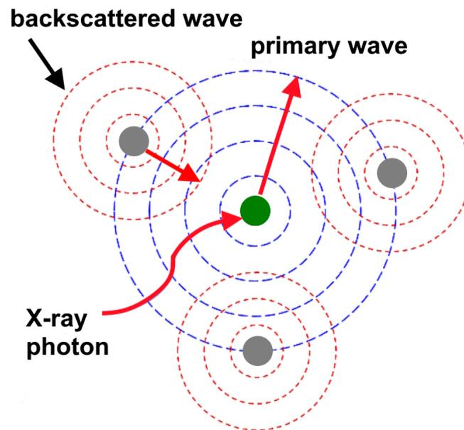
Figure 12. Schematic view of the formation mechanism of EXAFS oscillations [131].
