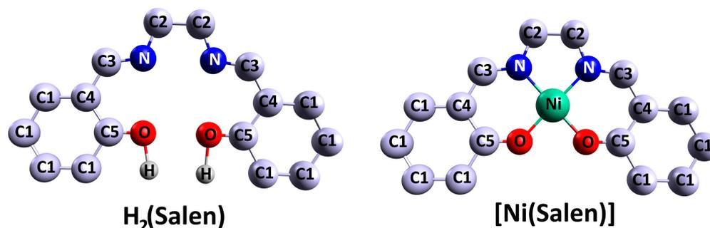
**Figure 1.** Schematic illustration of the  $H_2(Salen)$  salen ligand and  $[Ni(Salen)]$  molecular complex [46].
