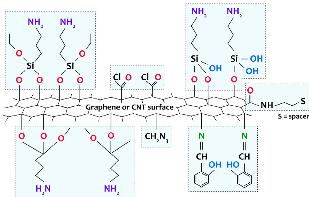
**Figure 5.** Representation of various groups covalently grafted to the surface of CNTs and graphene by amino-functionalization, chlorination, through spacer attachment, or through direct reaction of the ligand with the surface groups of the carbon support.
