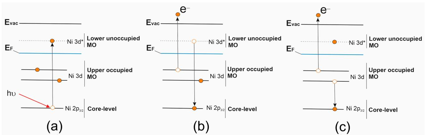
**Figure 10.** Schematic representation for resonant core electron excitation process (a) and Auger electron decay processes of a resonant excitation: (b) participator-Auger (*pA*) electron decay and (c) spectator-Auger (*sA*) electron decay [53].
