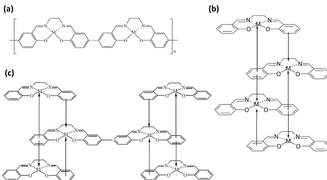
**Figure 2.** Models of poly-[M(Salen)] structure: (a) chain-like structure; (b) stack-like structure; and (c) hybrid variant.
