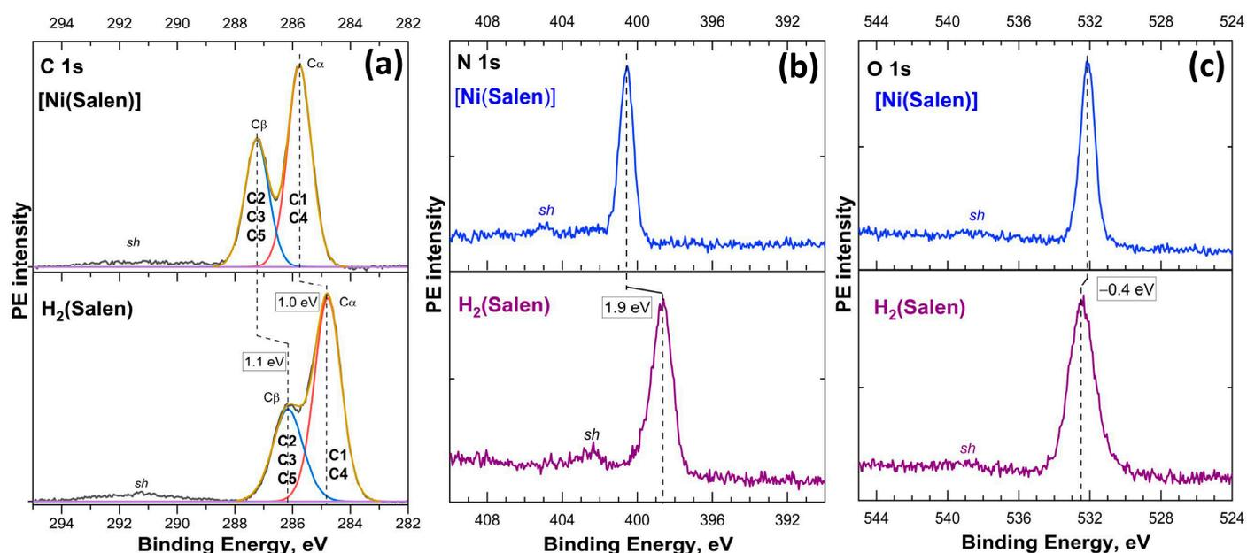
**Figure 14.** C 1s (a), N 1s (b), and O 1s (c) photoelectron spectra of the H<sub>2</sub>(Salen) molecule and [Ni(Salen)] complex measured using Al K $\alpha$  radiation ( $h\nu = 1486.6$  eV) and plotted on the scale of electron binding energies relative to the Fermi level [46].
