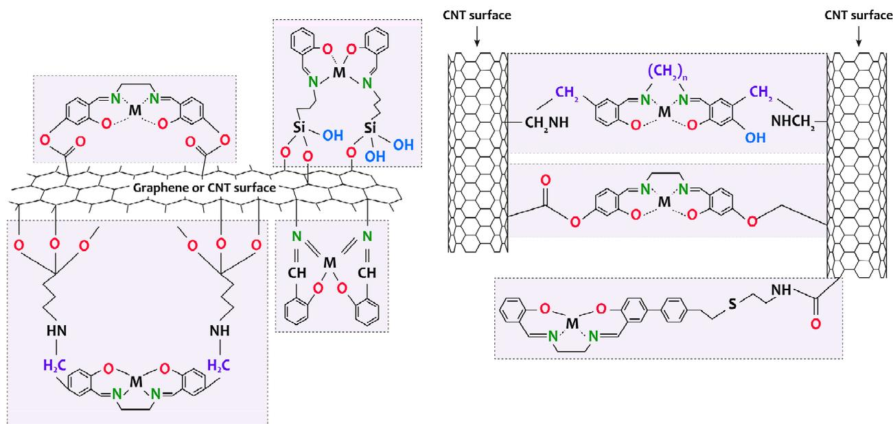
**Figure 6.** Schematic representation of the formation of [M(Salen)]/carbon nanotubes and [M(Salen)]/graphene composites.
