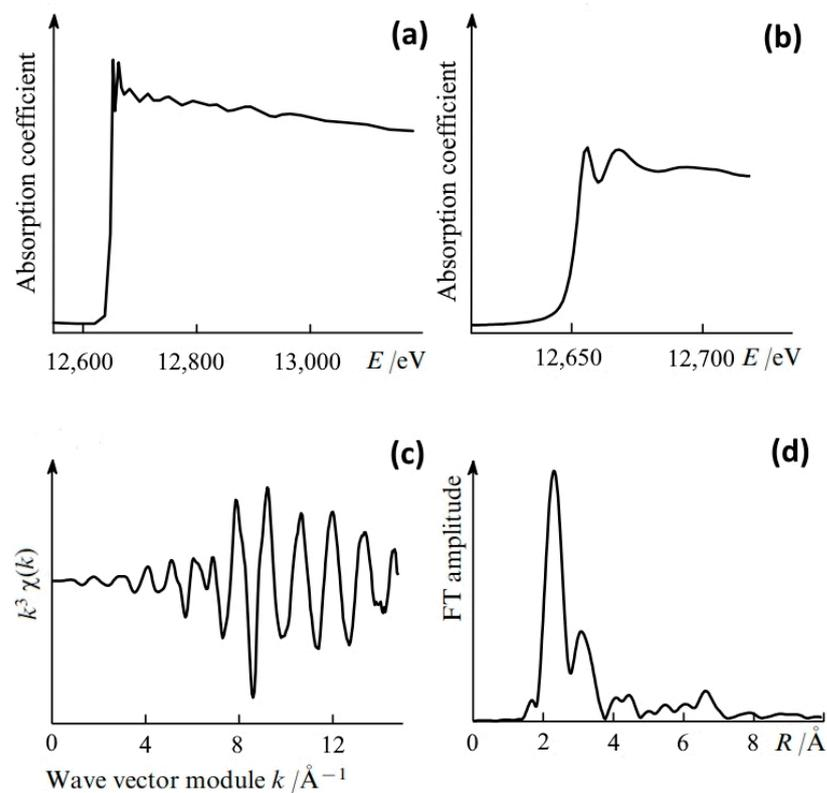
Figure 13. Steps of EXAFS data processing: (a) an experimental X-ray absorption spectrum; (b) the amplified NEXAFS region; (c) the normalized EXAFS curve (the oscillating part of the X-ray absorption coefficient); and (d) the Fourier transform (FT) of the normalized EXAFS curve; the maxima of the Fourier transform correspond to the coordination spheres around the central atom [129].
