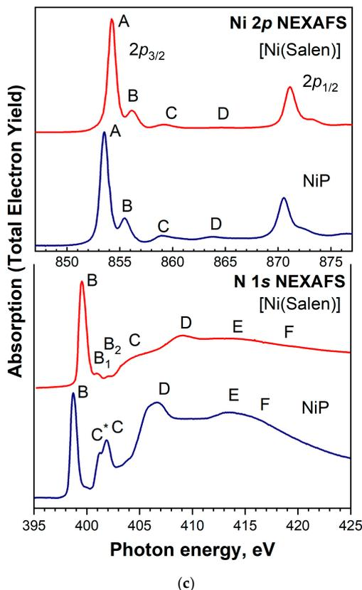
**Figure 11.** (a) X-ray absorption spectrum with regions corresponding to NEXAFS and EXAFS, and (b) schematic representation of NEXAFS mechanism due to multiple scattering. (c) Ni  $2p_{3/2,1/2}$  and N  $1s$  NEXAFS spectra of [Ni(Salen)] compared to the corresponding spectra of nickel porphyrin NiP [45].
