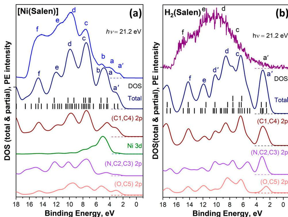
**Figure 15.** Comparison between experimental valence band and DOS spectra that were from DFT calculations for [Ni(Salen)] complex (a) and H<sub>2</sub>(Salen) (b). Vertical black bars show the energy positions of valence molecular orbitals, which have been broadened by Gaussian lines with a full width at a half maximum of 1 eV. The lowercase letters a', a, b, c, d, e and f denote the photoemission signals of individual sub-bands of the valence band [46].
