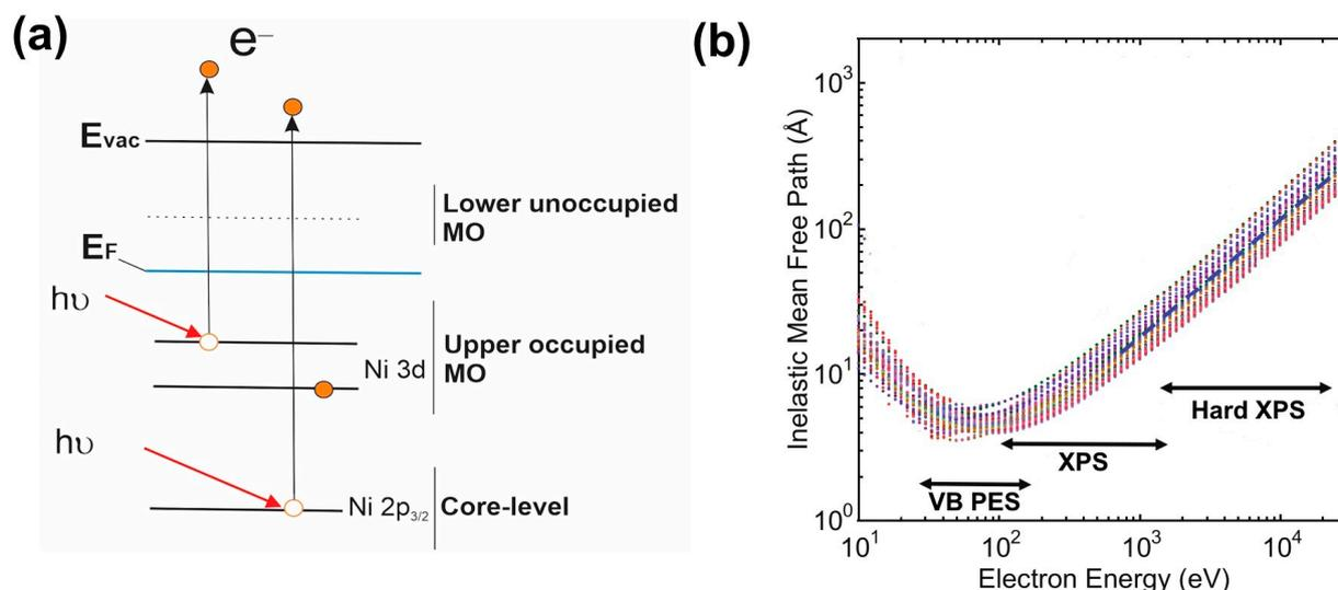
**Figure 7.** Schematic representation of the photoionization process (core or valence electron) (a) and energy dependence of inelastic mean free path  $\lambda$  of photoelectrons calculated for the 41 elements from the often-used formula TPP-2 M (adapted from Ref. [120] with permission) (b).
