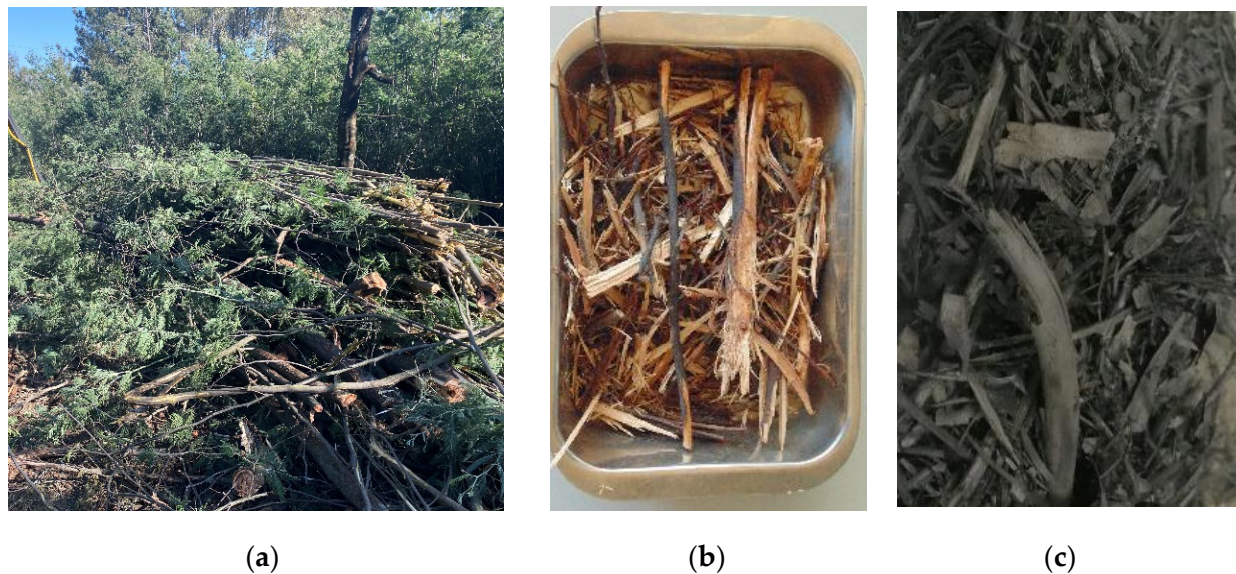
Figure 3. A. dealbata (a) waste material in the forestry, (b) crushed material, and (c) final biochar.
